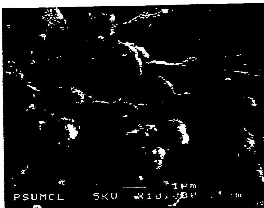
Figure 37. FESEM micrograph of oxidative deposits on stainless steel from a jet A fuel, 10,000x.
