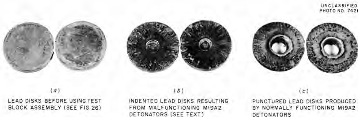
Fig. 24. Illustration of Typical Results from Normally and Abnormally Functioning M19A2 Detonators on Lead Disks Used in Puncture Tests.
