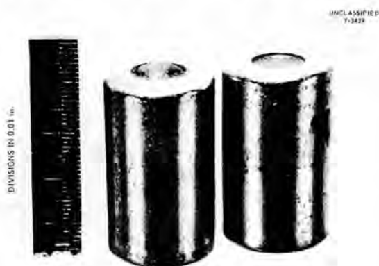
Fig. 24. Illustration of Typical Results from Normally and Abnormally Functioning M19A2 Detonators on Lead Disks Used in Puncture Tests.
