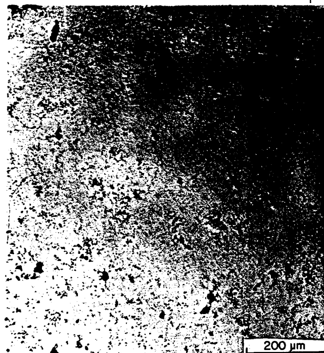
Figure 6 - Optical microstructure of Fe 3 Al obtained by hot-pressing of iron and aluminum powders.
