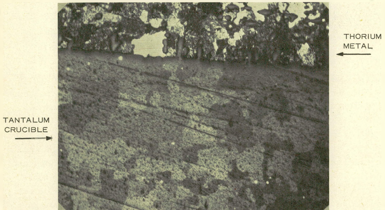
Fig. 6. Contact Area Molten Th Contained in Ta (Dark Field)
