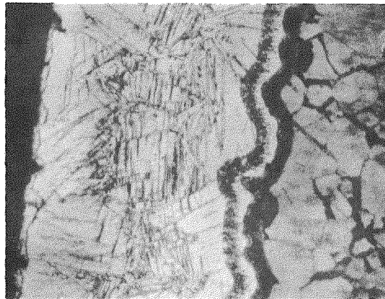
Microstructure of fuel pin No. 18692 removed from subassembly M099. Zirconium clad shows a metallographically estimated 2500 ppm hydriding, vacuum fusion analysis shows 700-900 ppm hydriding.
