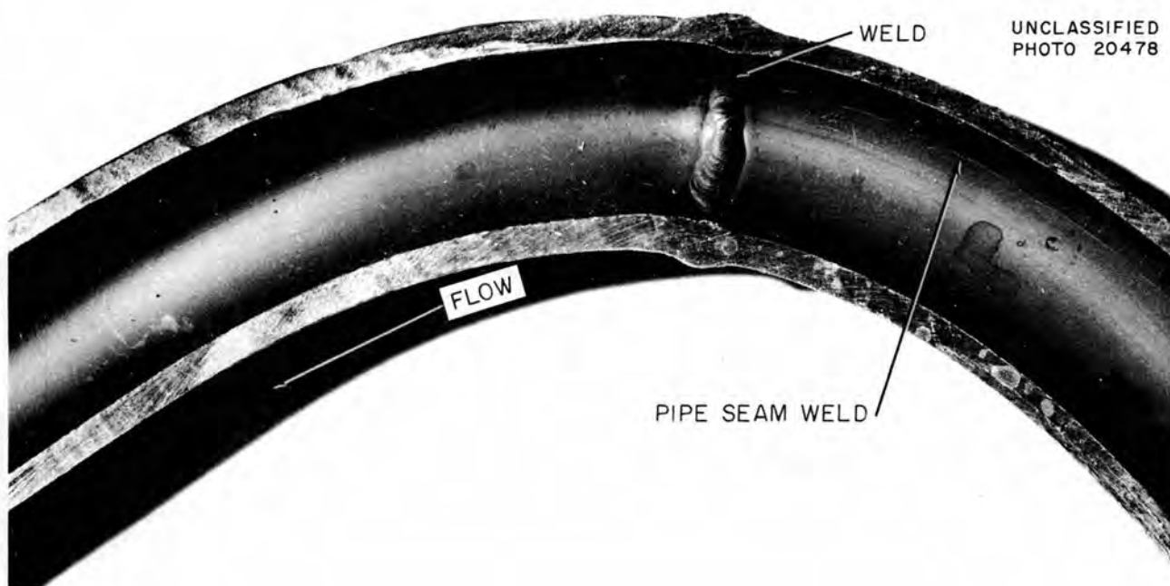
Fig. 39. Ninety-Degree Bend and Weld, Loop I.
