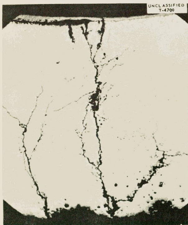
Fig. 88. Transgranular Cracks in \frac{3}{8} -in. Type 347 Stainless Steel Tube from Dynamic Corrosion Loop C. The inside (uranyl sulfate side) of the tube wall is at the top of the photomicrograph. 50X. Reduced 31%.
