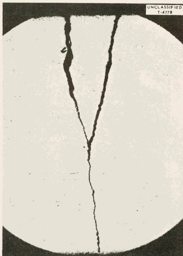
Fig. 90. Transgranular Cracks in 0.5-in. Type 347 Stainless Steel Tube from Dynamic Corrosion Loop C. The uranyl sulfate side of the tube wall is at the top of the photomicrograph. 50X. Reduced 32%.
