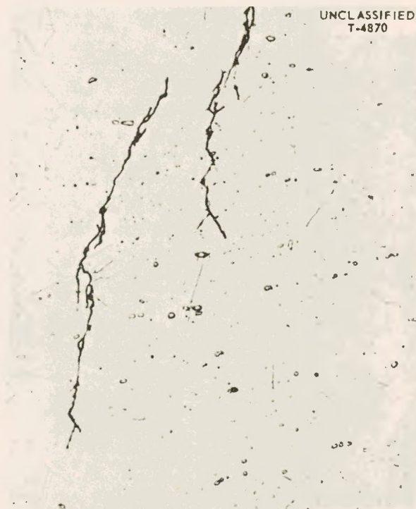
Fig. 91. Transgranular Cracks Adjacent to Main Crack in 0.5-in. Type 347 Stainless Steel Tube from Dynamic Corrosion Loop C. 750X. Reduced 11%.
