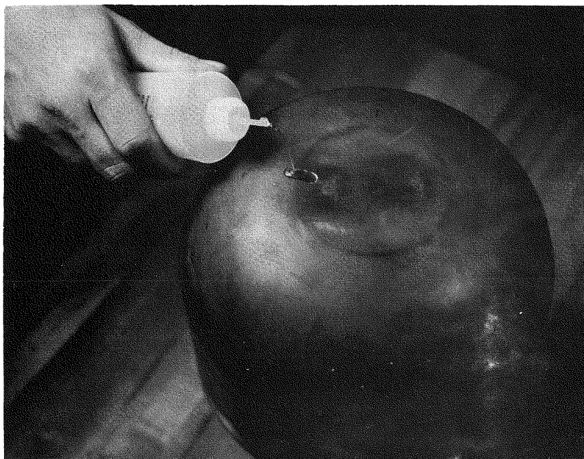
Figure 3-19. Leak Checking Inner Shell (Internally Pressurized)
