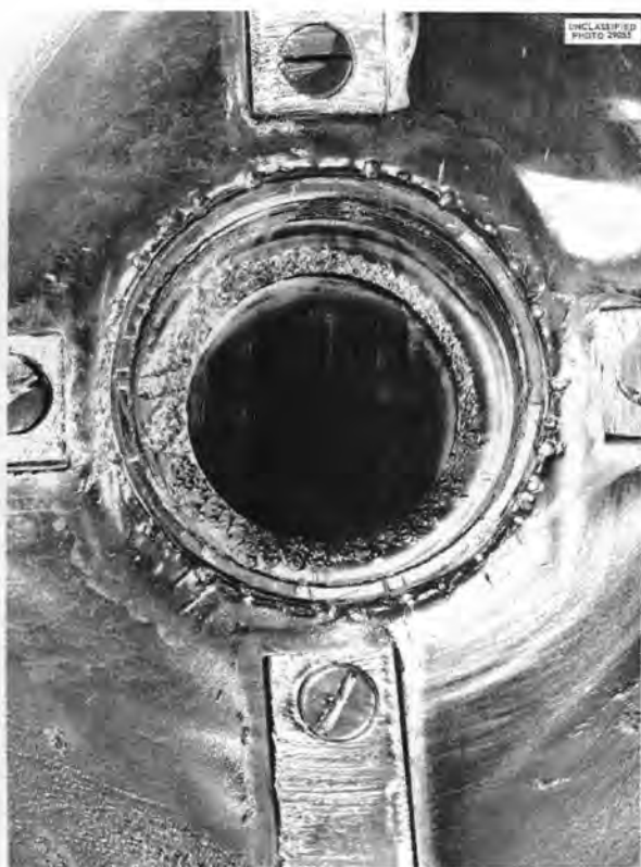
Fig. 13.3. Attack on Pump Suction Line; Slurry Run CS-35.
