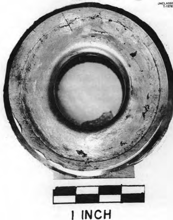
Fig. 5.2. Pitting Attack on Low-Pressure-Valve Bellows Head.
