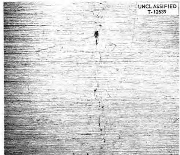
Fig. 12.3. Superficial Cracks on Type 347 SS Stressed at 15,000 psi After 2500 hr in Boiling, Aerated Uranyl Sulfate Solution Containing 100 ppm Bromide. 5X. Reduced 13%.
