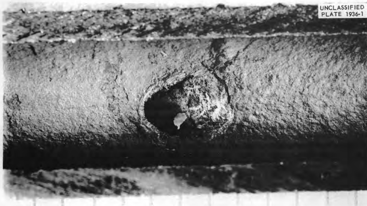
Fig. 3.2. Tube Failure in HRT Mockup Heat Exchanger.
