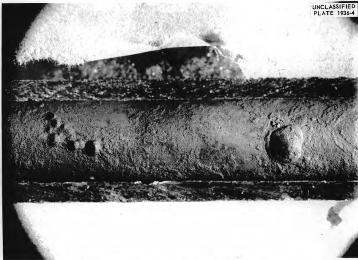
Fig. 3.3. Typical Pitting in Tubes of HRT Mockup Heat Exchanger.
