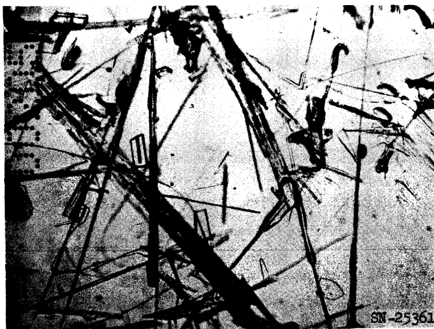
Fig. II-2. Growth of BeO single crystals.
