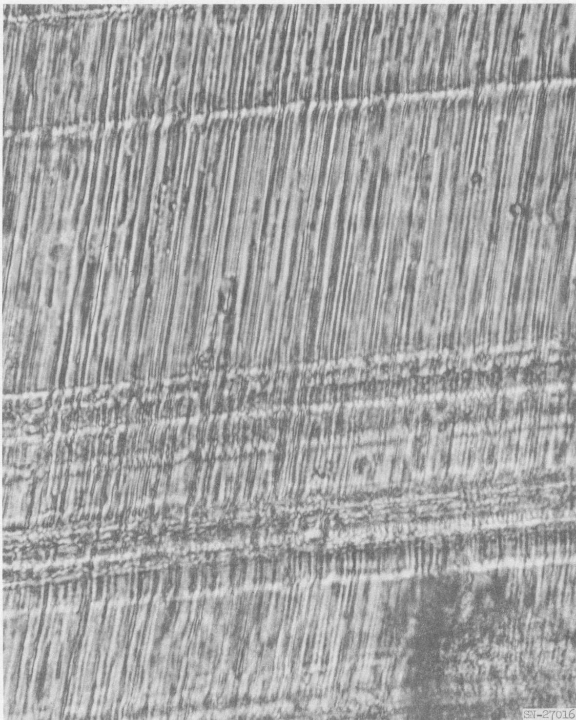
Fig. II-4. Photomicrograph of a portion of the crystal in Fig. II-3 showing both sets of striae. Polarized light, 152 \times .
