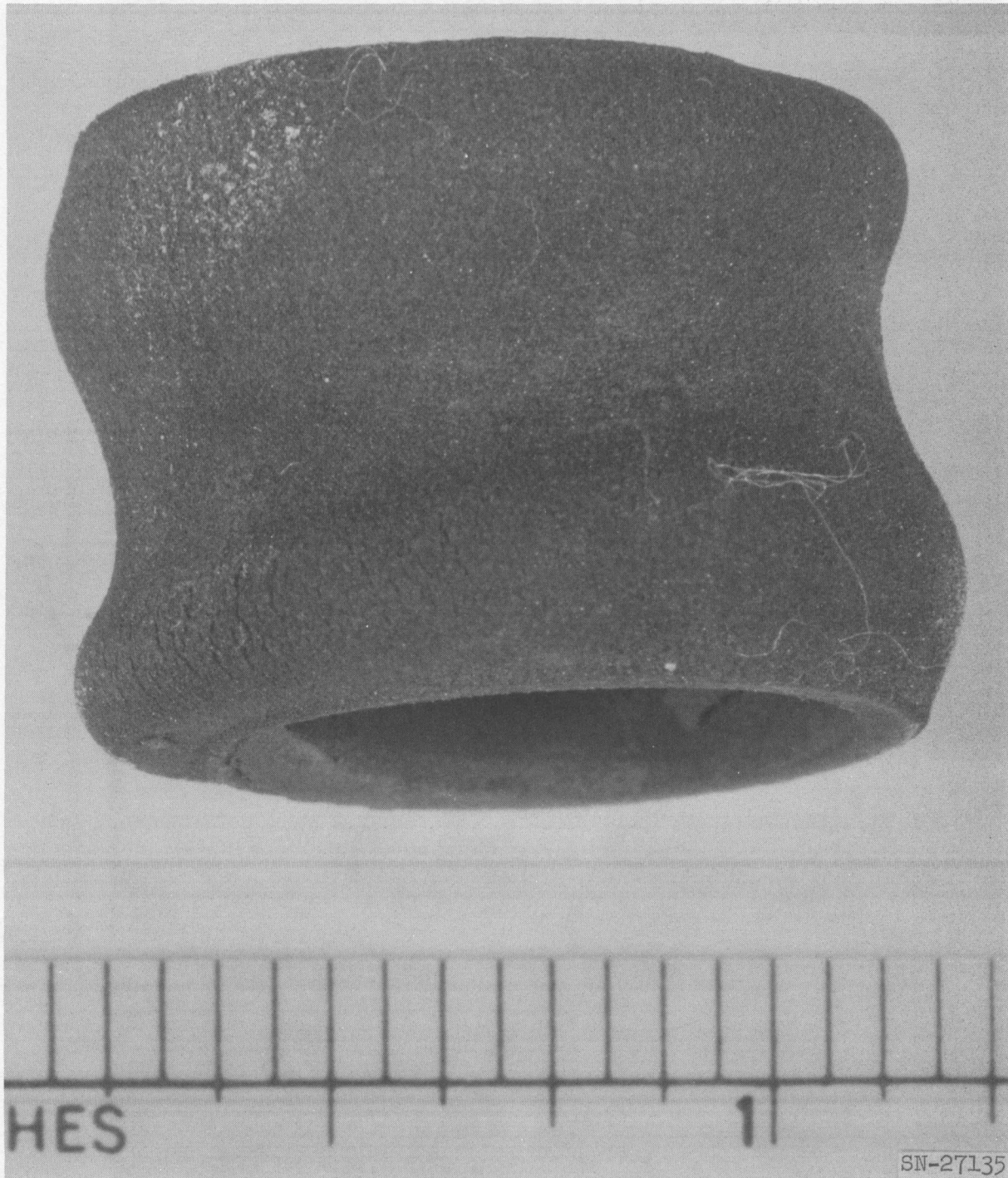
Fig. V-11. Chrome Cerametalix tube after testing at 2500°F under compressive stress of 2200 psi.
