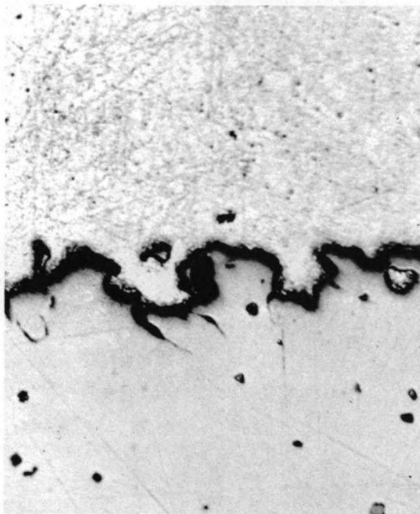
Fig. 19. Absence of a Diffusion Layer in the Couple Uranium-Magnesium After 16 Hours at 600°C.
