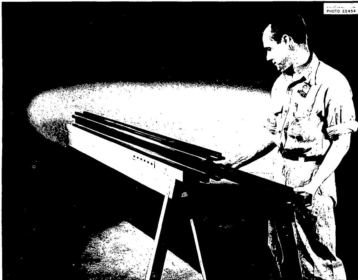
Fig. 29. Full-Size Model of Four Moderator Blocks and One Fuel-Unit Assembly Made of High-Density Graphite.
