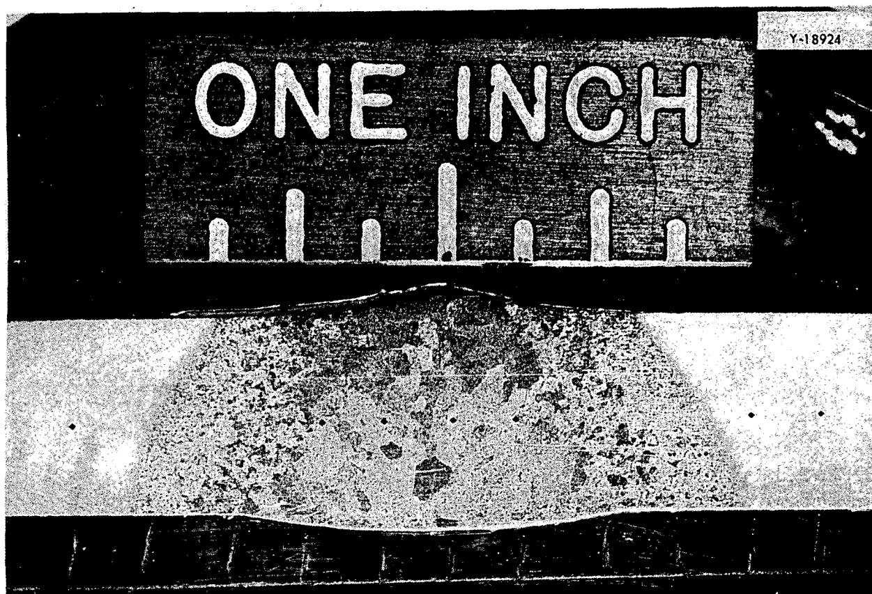
Fig. 14.5. Macrograph of Zircaloy-2 Weld Showing Rapid Change in Structure. Oblique Lighting.
