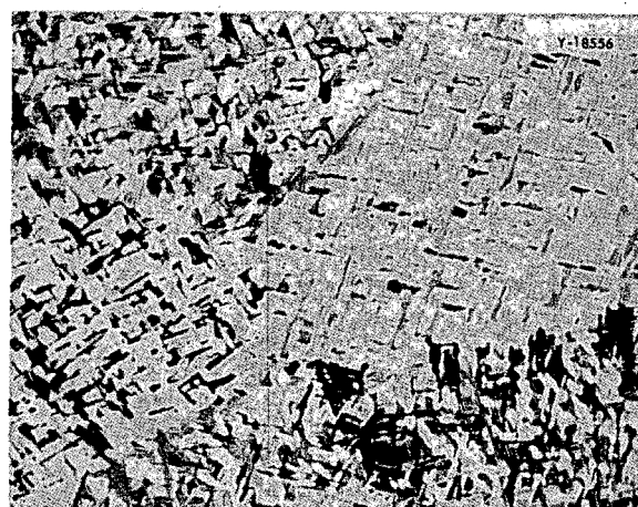
Fig. 14.4. Deposited Weld Metal Showing Coarse Transformed Beta Grains. Polarized light, 100X. Reduced 31%.
