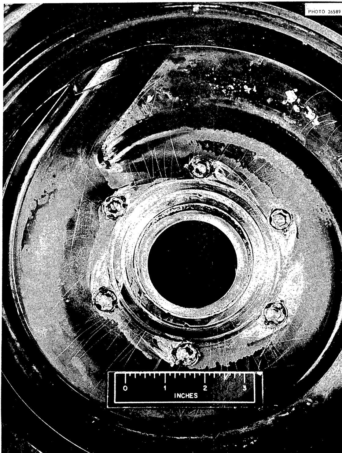
Fig. 9.10. 200A Pump Volute Showing Areas of Attack During Run 200A-5B.
