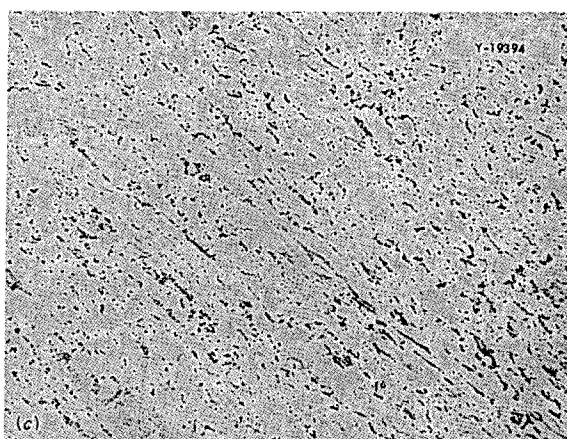
Fig. 14.7. Ti-6% Al-4% V Specimens Exposed in Recombiner Loop. (a) Recombiner specimen RL-1. (b) Cell specimen CL-3. (c) Control specimen RL-1C. 500X. Reduced 32%.
