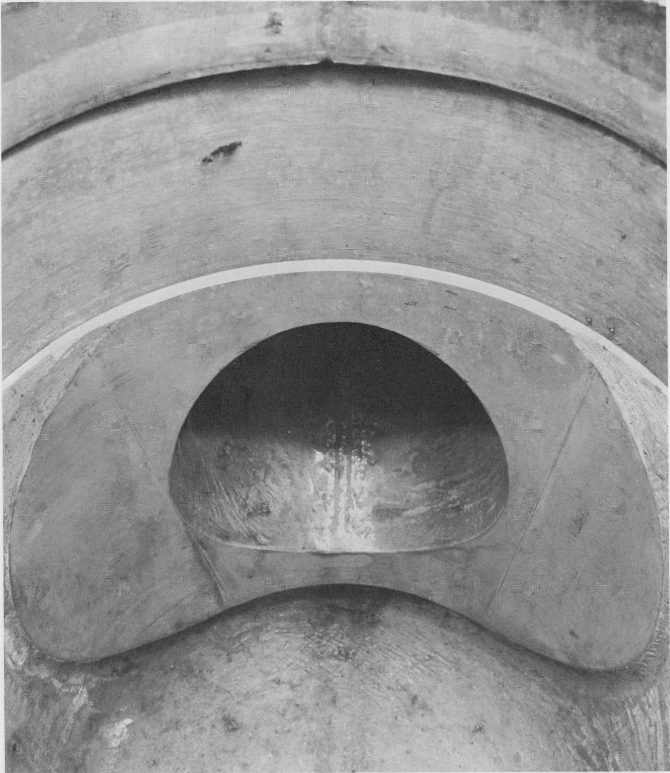
Fig. 20. Seat Surface of the 6-in. Round Port Production Valve after two Water Baths and one Steam Bath
