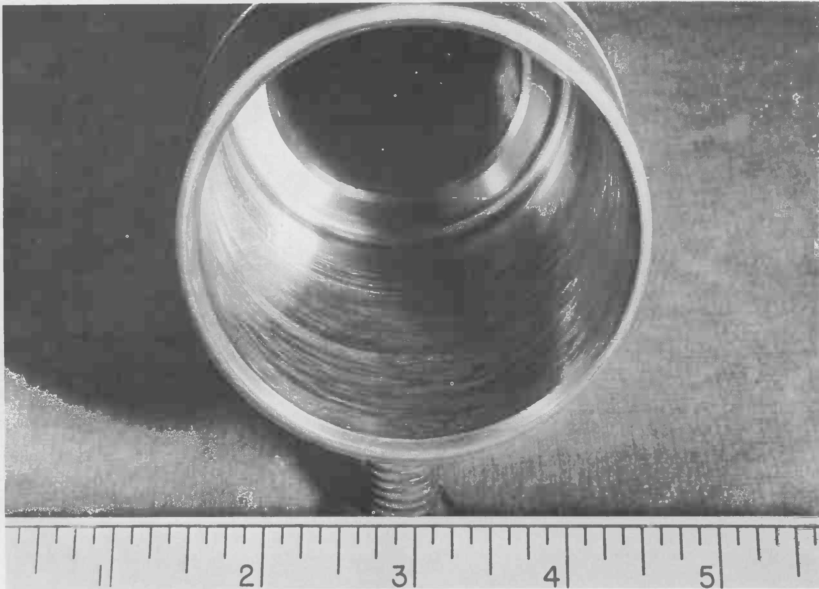
Fig. 36. Center Shield Ring (showing galling damage)
