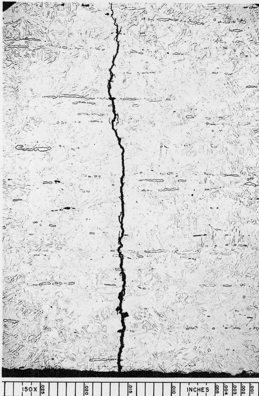
Fig. 12. Stress-Corrosion Crack in a 17-4 PH Stress Specimen Exposed 14,364 hr in the Vapor above HRT Solution at 300°C. (T13938)
