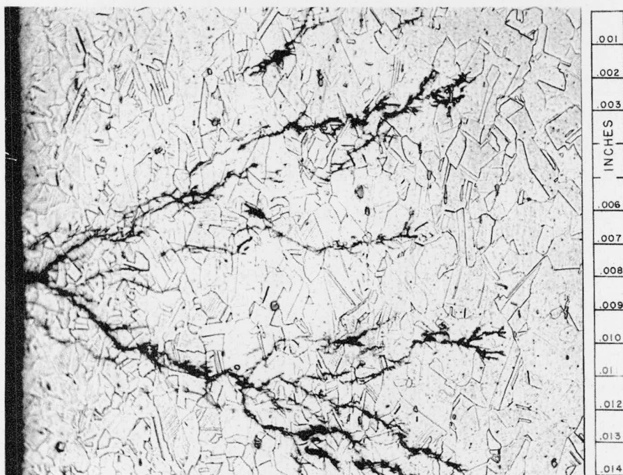
Fig. 13. Photomicrograph of Stress-Corrosion Cracking in Annealed Type 304 Stainless Steel After 100-hr Exposure to Distilled Water Containing 100 ppm Chloride at pH 2.8. Magnification 250X. (T13919)
