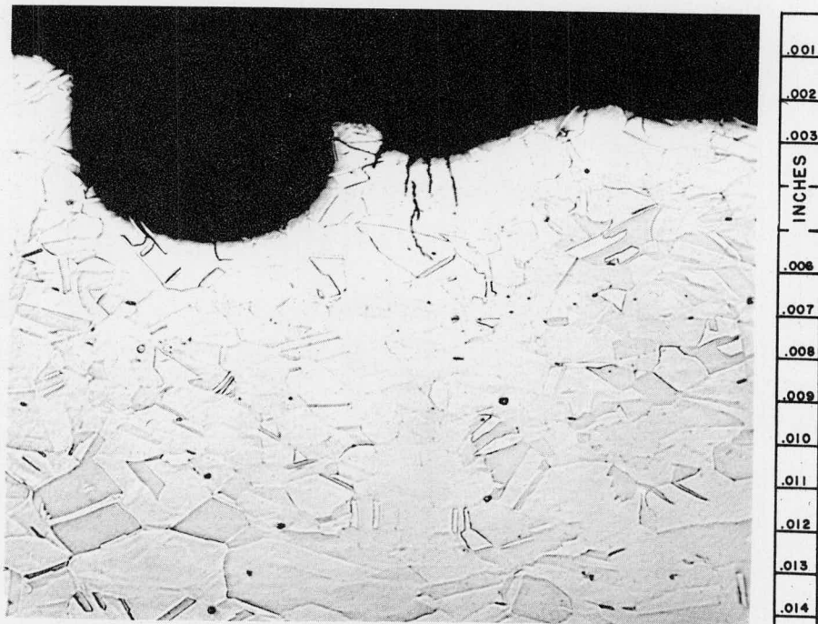
Fig. 16. Photomicrograph of Stress-Corrosion Cracking in Incoloy after 500-hr in Distilled Water at 300^\circ\text{C} Containing 100 ppm Chloride at pH 2.8. Magnification 250X. (T-13569)
