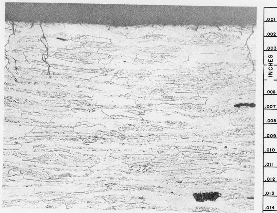
Fig. 15. Photomicrograph of Stress-Corrosion Cracks in Croloy 16-1 Stainless Steel after 100-hr Exposure to Boiling 42% \text{MgCl}_2 . Magnification 250X. (T13645)
