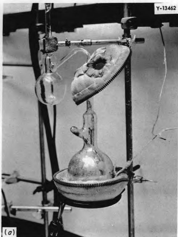
Fig. 8. Rubidium Distillation Vessel. (a) Impure rubidium sealed to distillation apparatus. (b) Impure rubidium ready for distillation.
