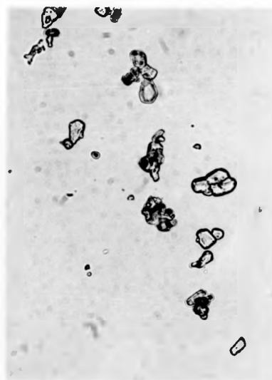
No. 3261-02, 160X Oven Dried, 36 hrs @ 66 C Plus 8 hrs @ 116 C, 1800 cm 2 /g
