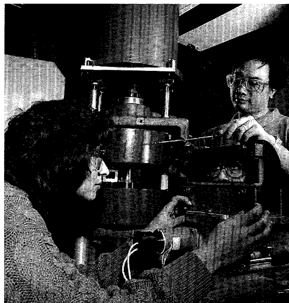
Figure V.6 At the IPNS, Argonne researchers adjust the polarized neutron beam by using the super mirror analyzer on the POSY reflectometer. POSY is used to study near-surface behavior such as magnetic multilayers and also bonding and diffusion in polymers.
