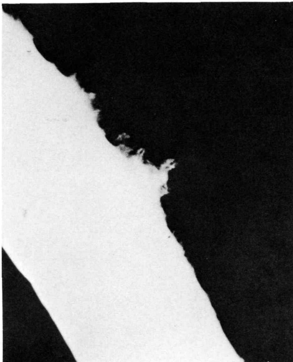
FIGURE 7. Microradiograph of NbC Bore Coating Near the Coater Inlet Showing Extensive Rooting Section Thickness: 0.008 in.
