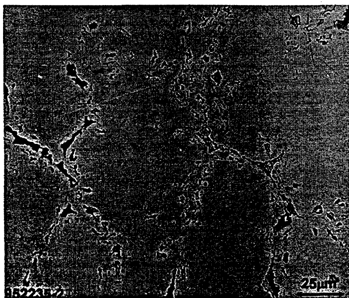
Fig. 3. Optical micrograph of centrifugally cast IC221M.
