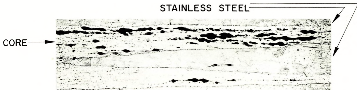
CUPPING OF CORE EDGE AT END OF CORE IN FUEL PLATE SEE SECTION "B"
