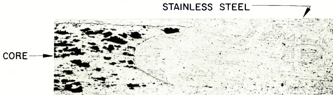
CUPPING OF CORE EDGE AT SIDE OF CORE IN FUEL PLATE; SEE SECTION "A"
