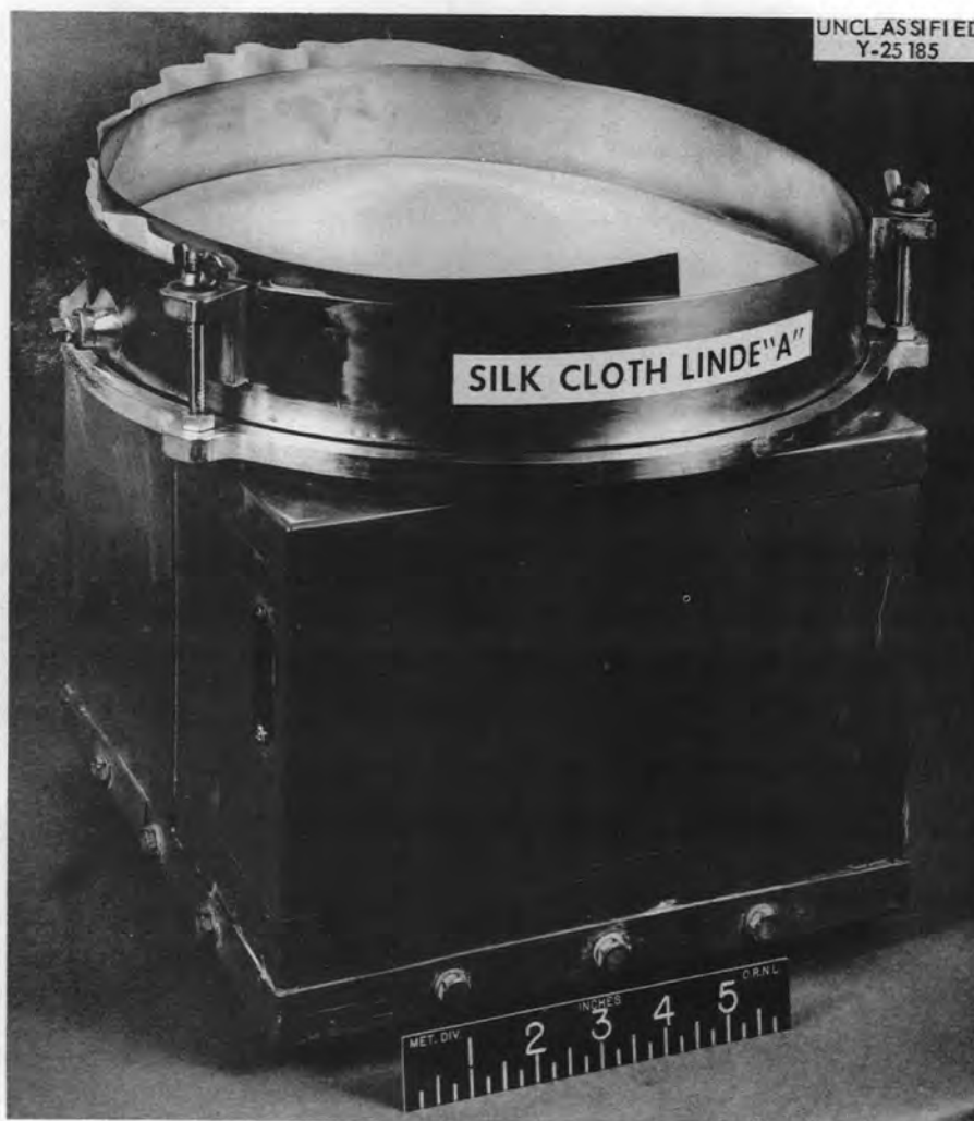
Fig. 4. Method Used for Securing Silk Cloth in Polishing Bowl with Expanding Spring-Steel Band.
