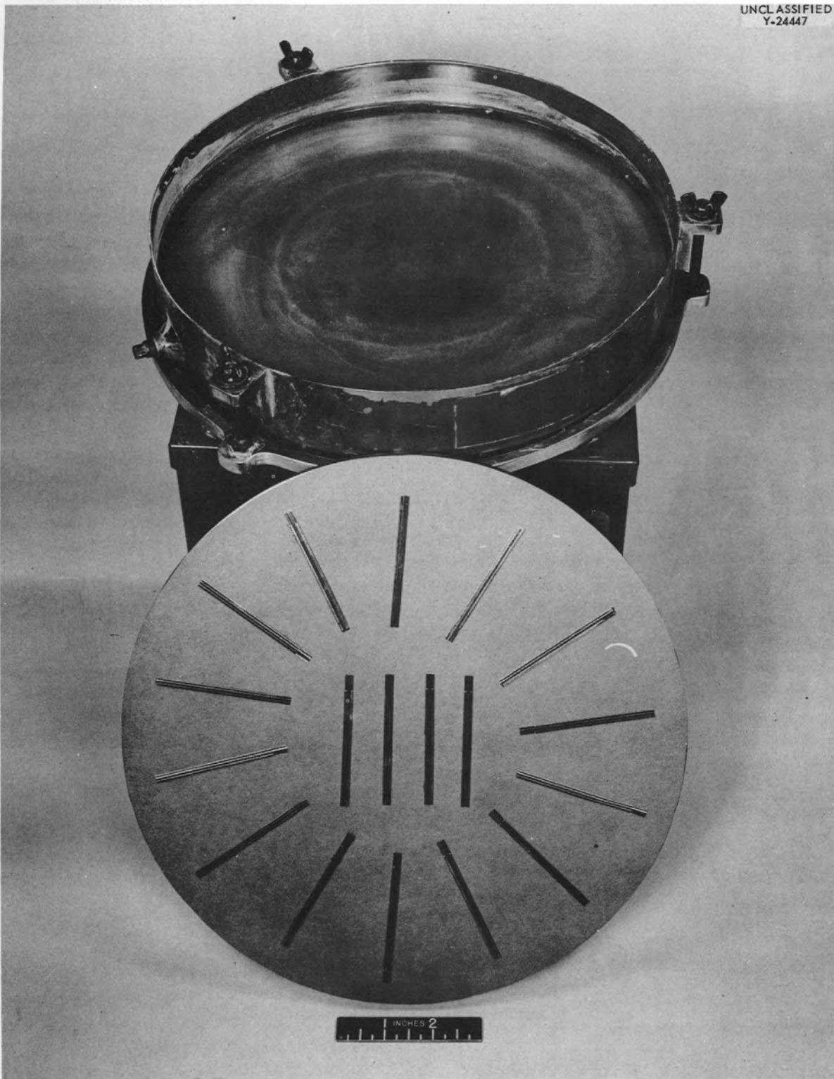
Fig. 11. Platinum-Gage Strips Cemented to a Weight Plate Prior to Being Placed in Vibratory Polisher.
