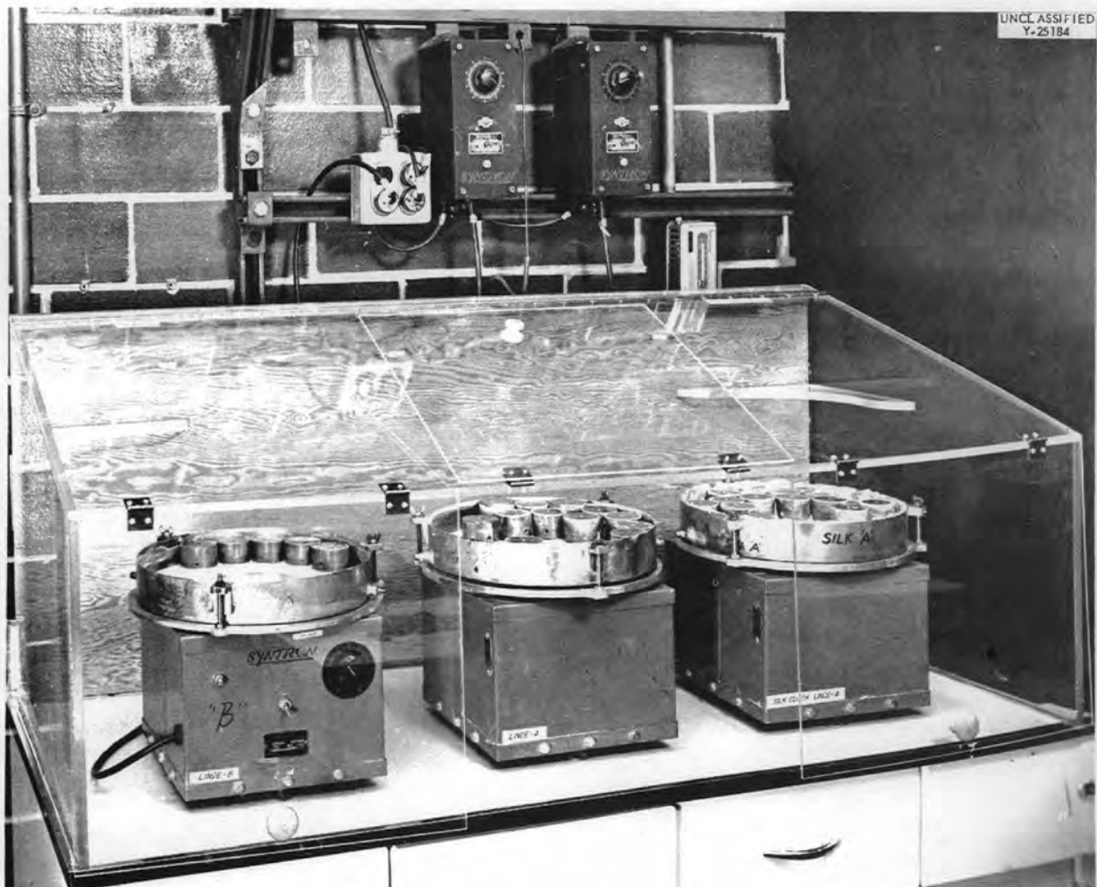
Fig. 5. The Arrangement of the Three Large Vibratory-Polishing Machines. Note that controls for the two polishers on the right are located outside and above the Lucite dust protector. The polisher on the left is the deep nap, Linde B bowl, the middle polisher is equipped with deep nap, Linde A, and the polisher on the right is equipped with silk, Linde A bowl.
