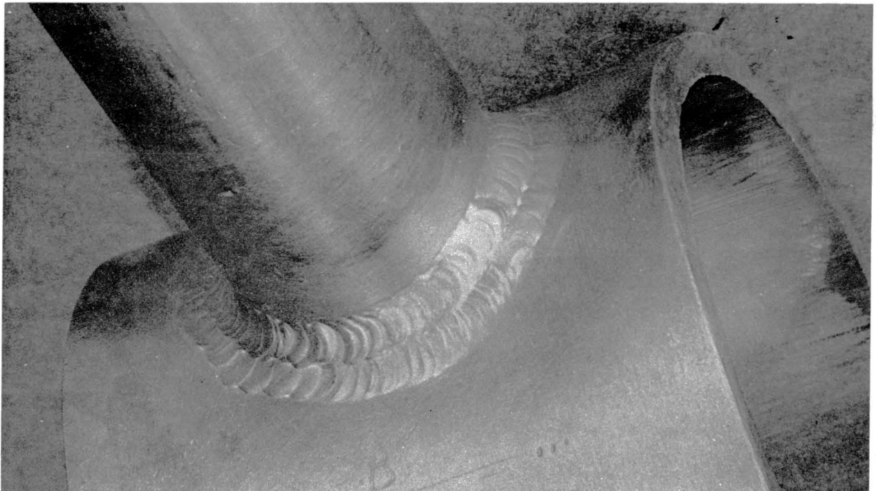
Fig. 2-4.5 — Corner welds. Top — nozzle outside. Bottom — nozzle inside.
