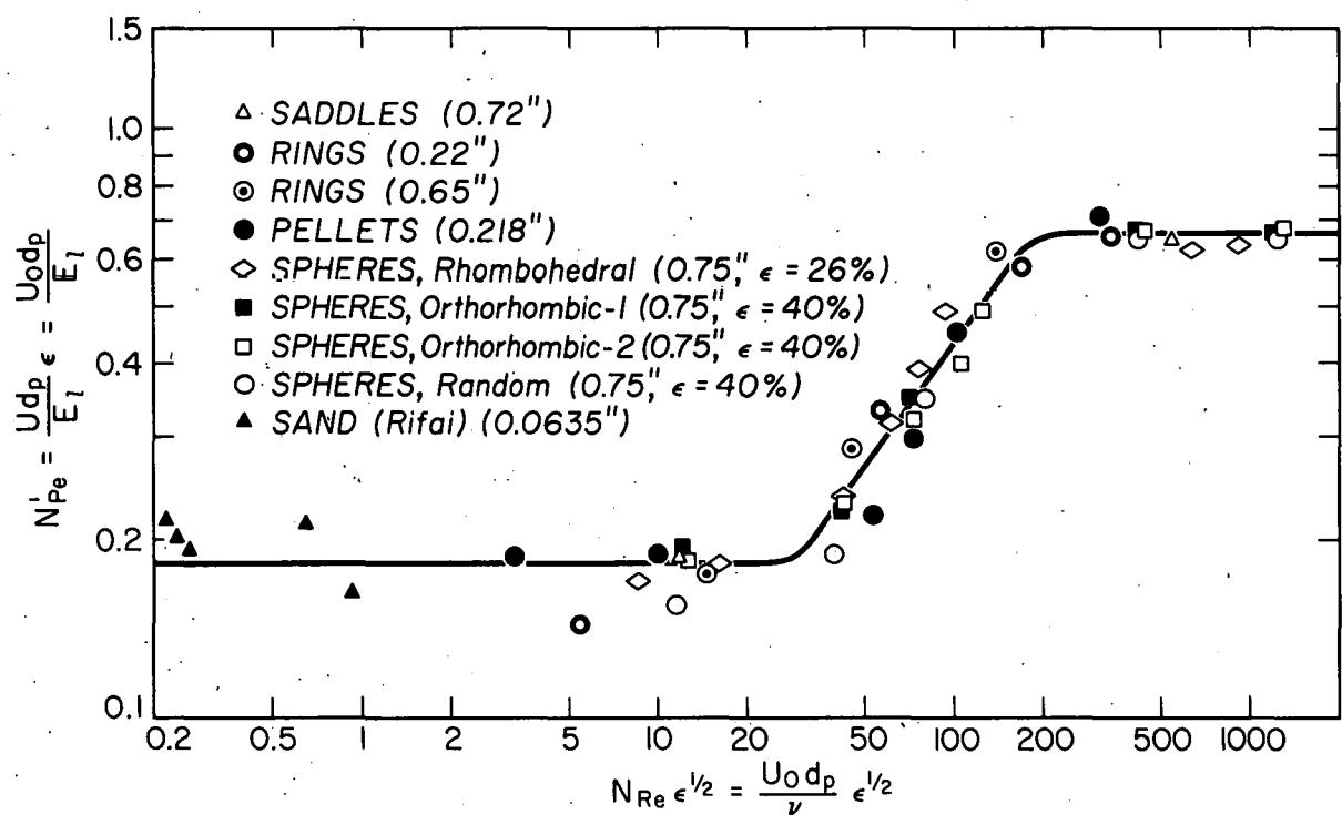
Fig. 35 Modified Peclet number for longitudinal dispersion in single-phase flow, as a function of Reynolds number.
