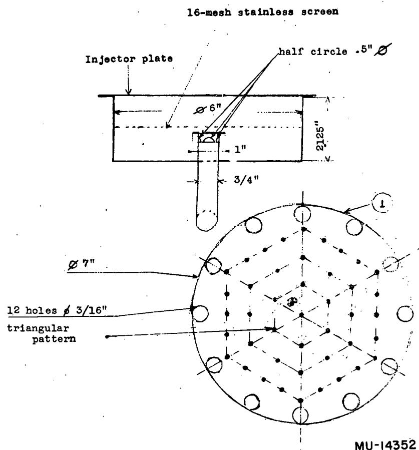
Fig. 21 Detail of nozzle construction.
