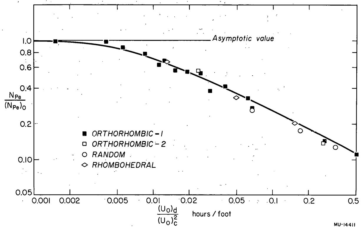
Fig. 5. Correlation plot for continuous-phase longitudinal dispersion.
