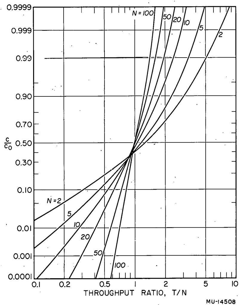
Fig. 3. Random-walk breakthrough concentration.
