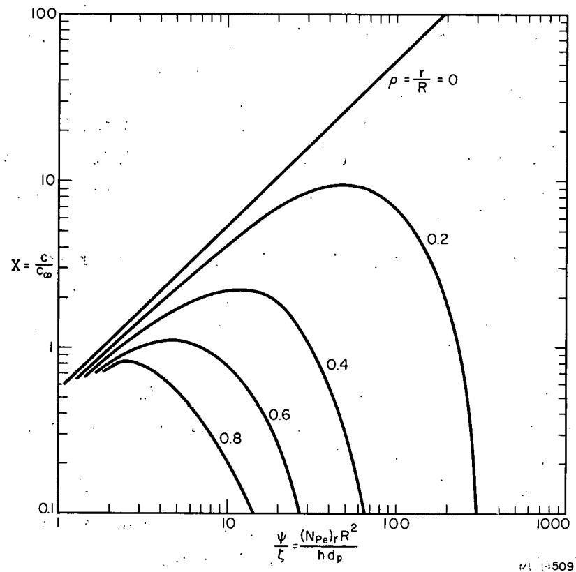
Fig. 6 Radial-dispersion function.
