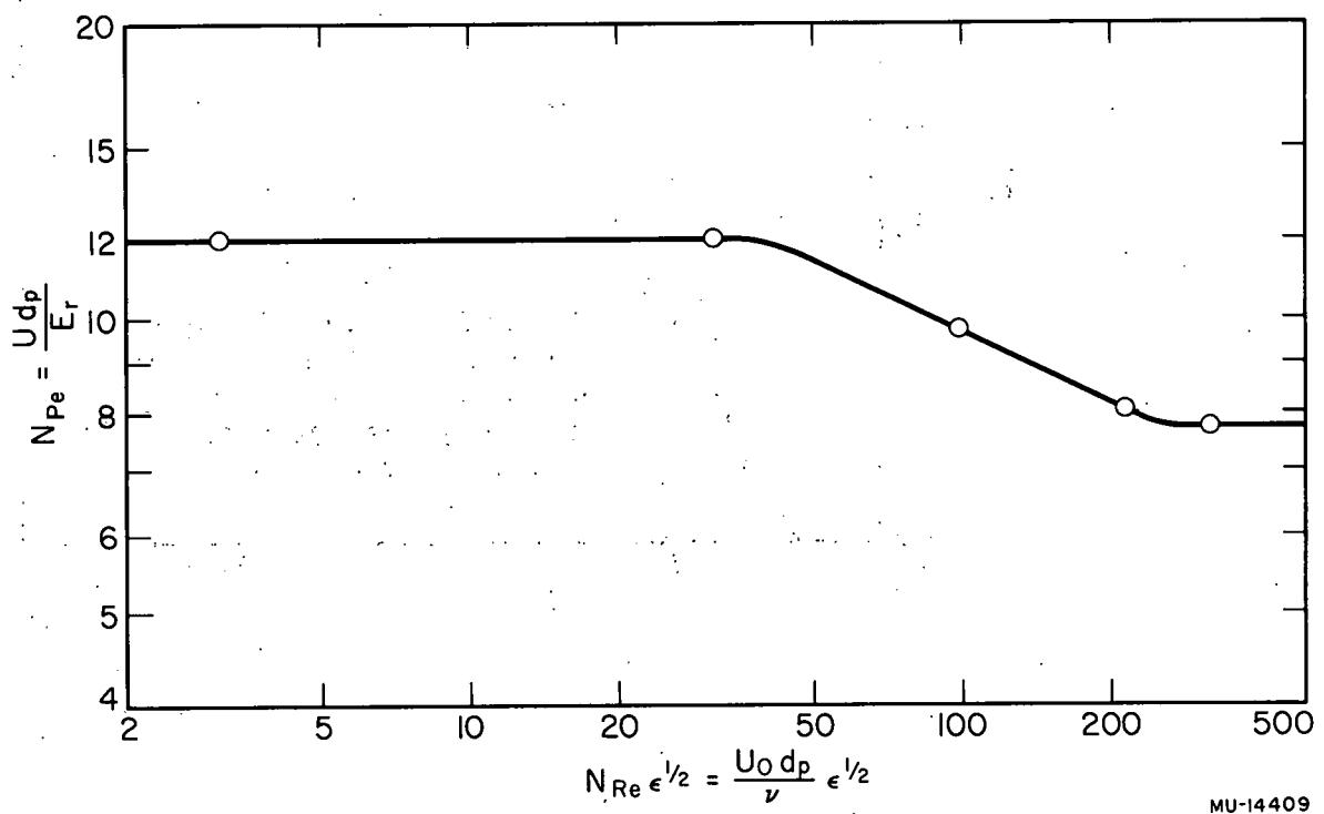
Fig. 37 Radial Peclet number as a function of Reynolds number
