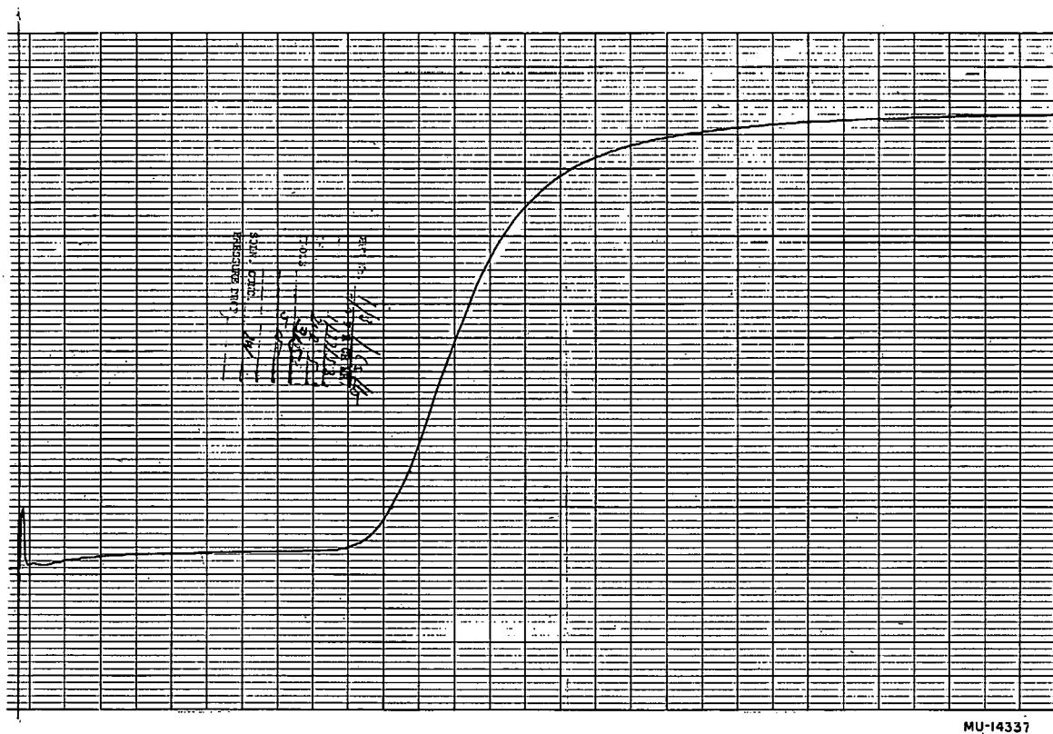
Fig. 32 Recorder chart for step-function breakthrough
