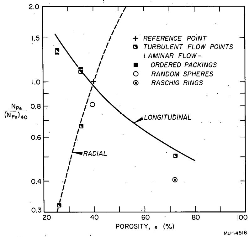
Fig. 36 Relative longitudinal Peclet number as a function of porosity.
