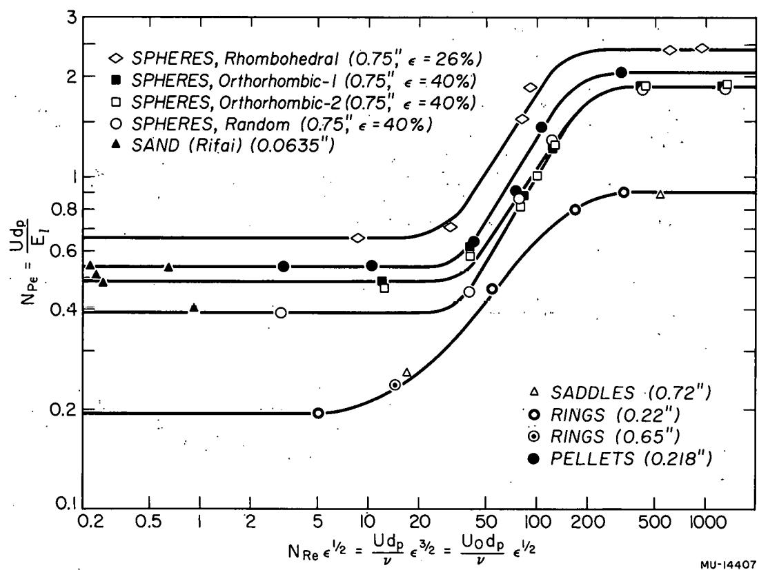
Fig. 34 Longitudinal Peclet number as a function of Reynolds number.
