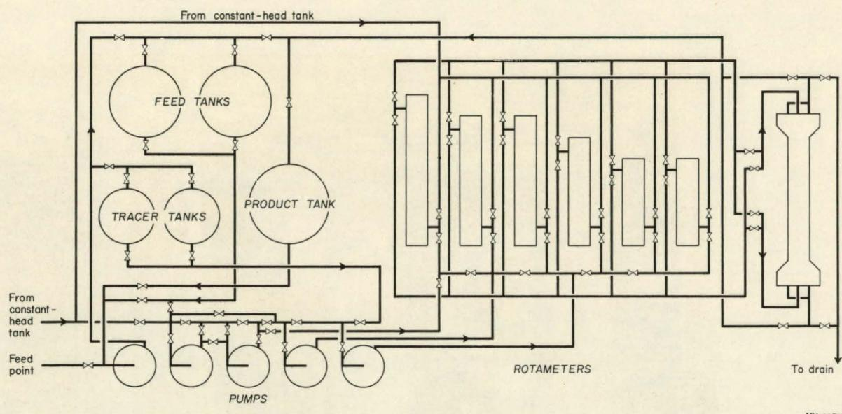
Fig. 28 Layout of flow system.
