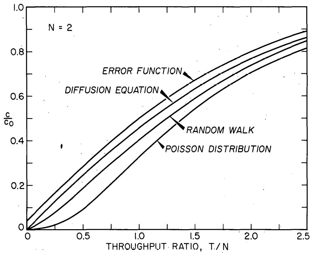
Fig. 1 Breakthrough curves given by various derivations ( $N=2$ ).
