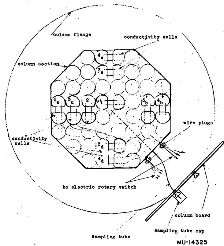
Fig. 13 Location of conductivity cells--Columns 1 and 2 (octagonal). The cells at each level were identified by the reference numbers shown.
