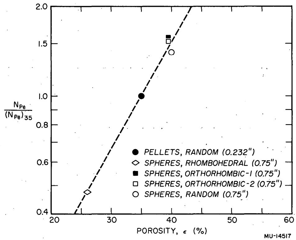
Fig. 38 Relative radial Peclet number in turbulent flow as a function of porosity.
