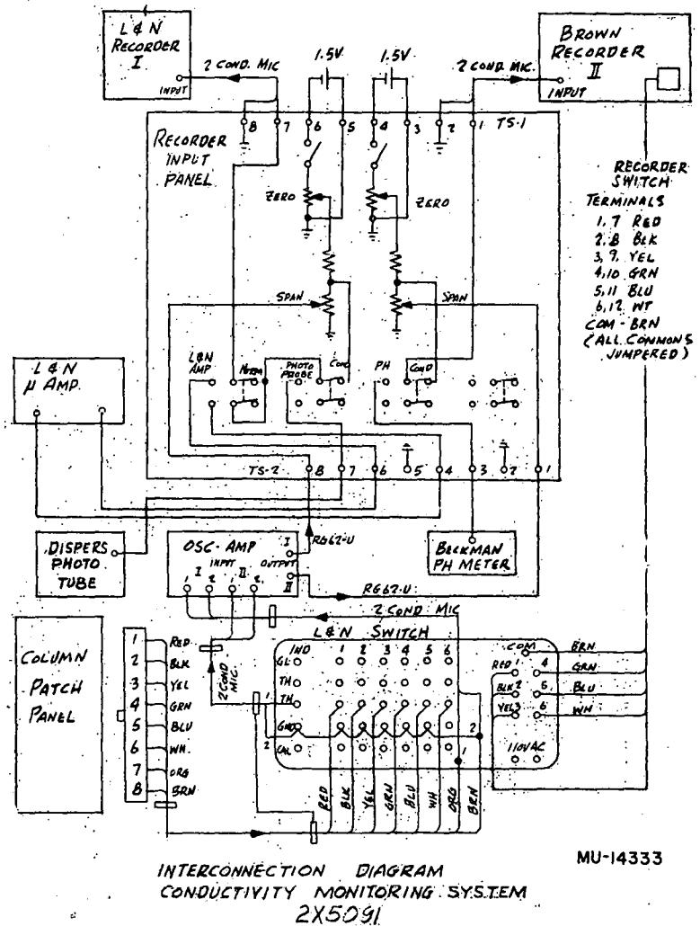
Fig. 25 Switching arrangement for conductivity recorders.
