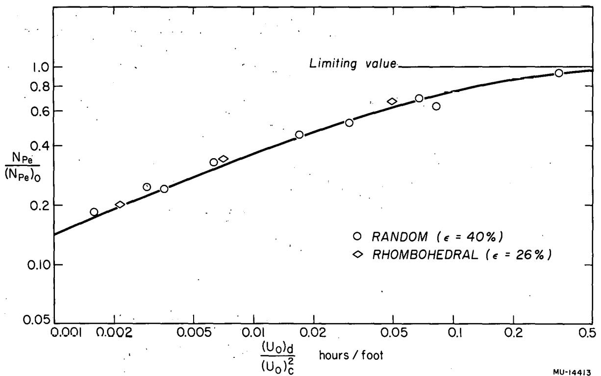
Fig. 10 Correlation plot for discontinuous-phase longitudinal dispersion for 0.75-inch spheres.
