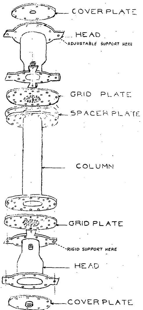
Fig. 20 Exploded assembly diagram of entire column.
