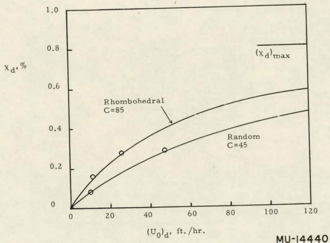
Fig. 13 Holdup of discontinuous phase for stationary continuous phase.
