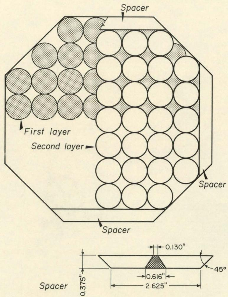
Fig. 9 Arrangement of packing and spacers, Column 1 (Rhombohedral).
