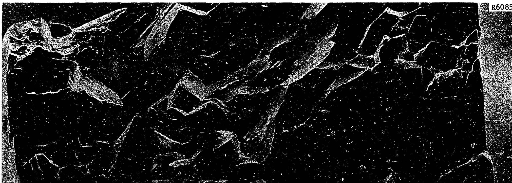
Fig. 5. Fracture Surface of Type 304 Stainless Steel Auger Specimen. The specimen was irradiated to 1 \times 10^{23} neutrons/cm 2 (>0.1 MeV) at 374°C and strained to failure at about 550°C in a vacuum of 2 \times 10^{-9} torr. The fracture is in excess of 90% intergranular. 500×. Reduced 13.5%.
