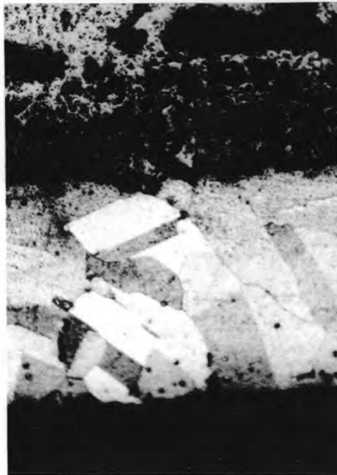
FIGURE 35 - SCOTT NiAl (-), 1800°F FOR 500 HOURS, 5 INCHES FROM HOT JUNCTION
