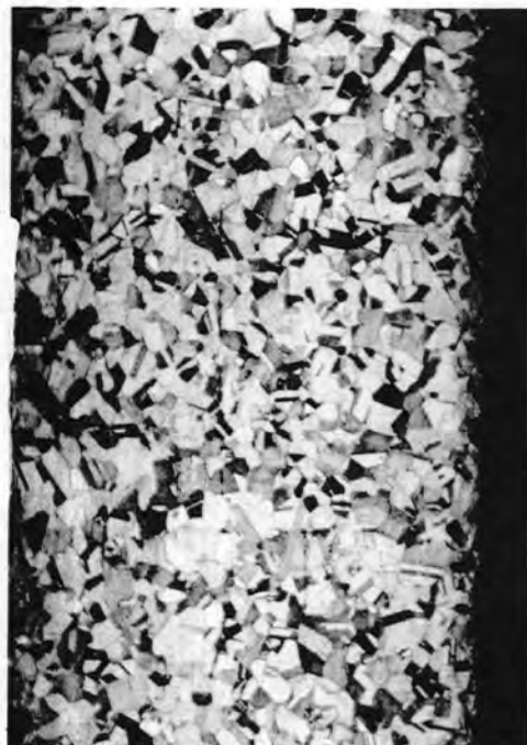
FIGURE 21 - AS RECEIVED HOSKINS ALUMEL
