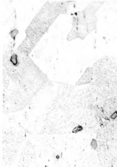
FIGURE 33 - ALUMEL IN SWAGED MgO ASSEMBLY - 5000 HOURS AT 1800°F
