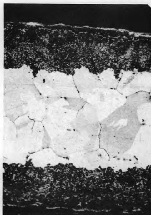
FIGURE 25 - ALUMEL, HOSKINS, EX- POSED 5000 HOURS AT 1300°F
