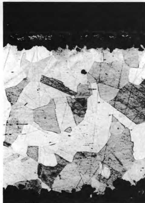
FIGURE 31 - ALUMEL IN SWAGED MgO ASSEMBLY - 5000 HOURS AT 1300°F
