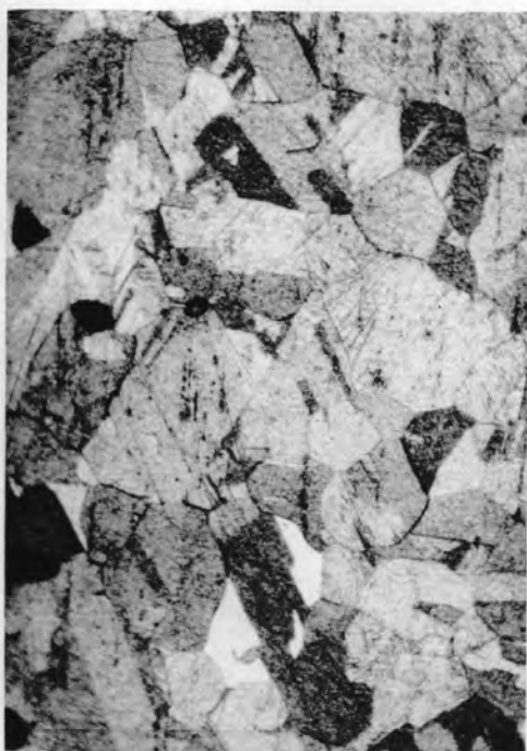
FIGURE 24 - CHROMEL, HOSKINS, EX- POSED 5000 HOURS AT 1800°F
