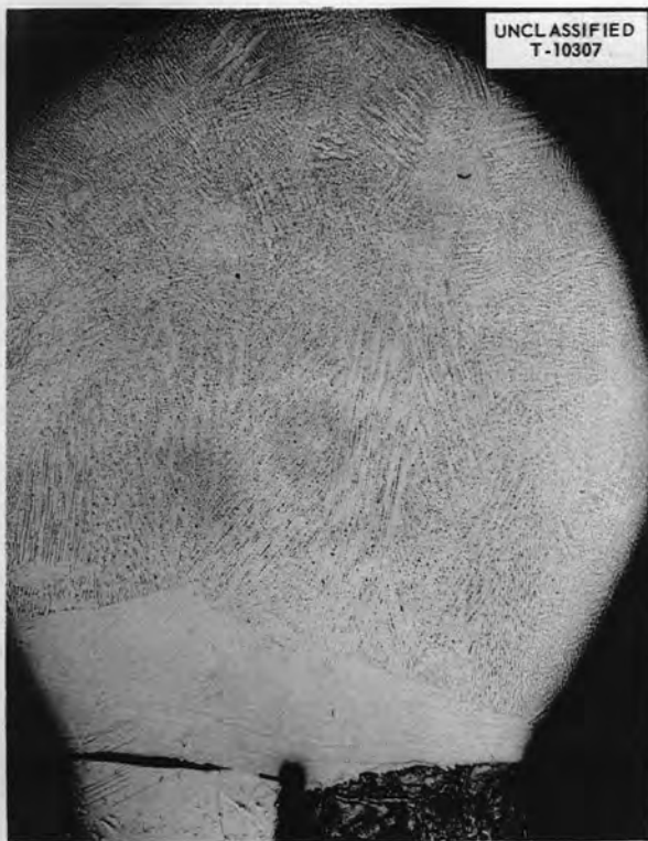
Fig. 118a. Cross Section of Heliarc-Welded Inconel-Coated Thermocouple Junction of No. 20 AWG Chromel and Alumel Wires. Note chromium oxide deposits in Chromel wire.
