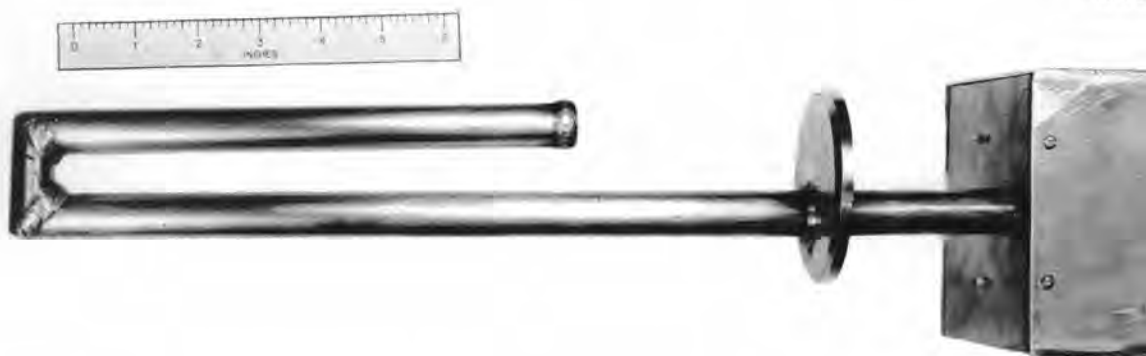
Fig. 100. Continuous-Monitor Type of Level Probe for Top-Mounting in NaK Pump Bowls.
