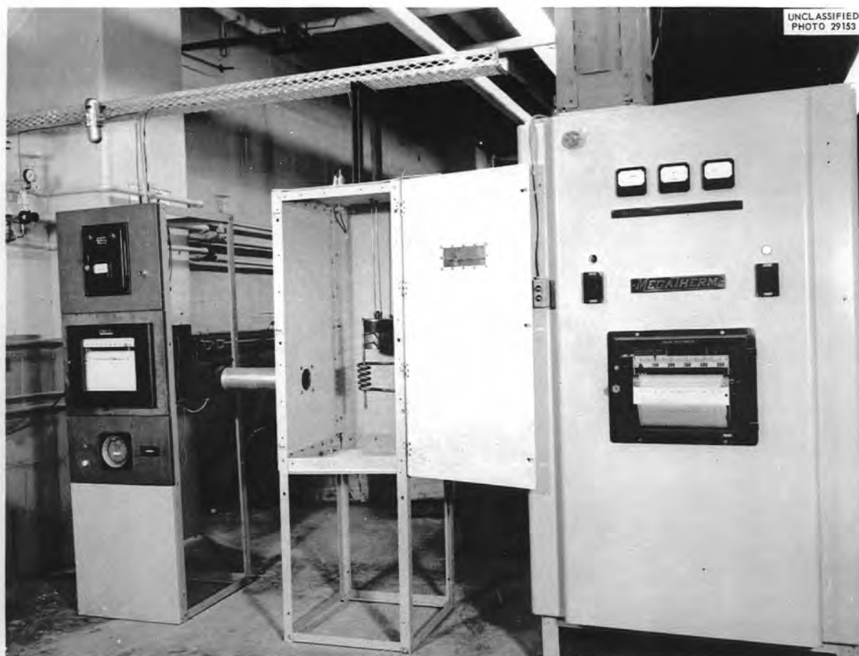
Fig. 116. Induction-Heating Facility for Rapid Heating Tests on Sheathed Thermocouples. Shows control instrument cabinet, test-specimen cabinet with coil, and main control cabinet.
