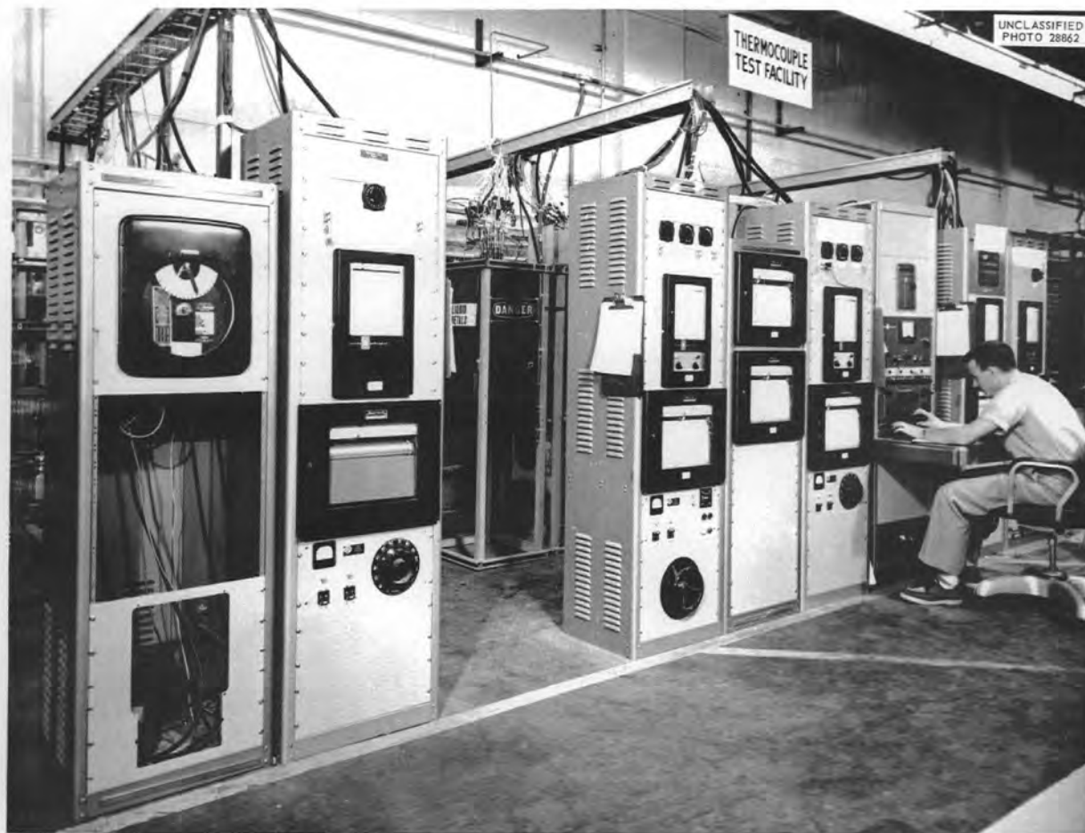
Fig. 114. Facility for Thermocouple Drift Testing and Calibration. Shows furnace with sheathed couples, five furnace-control cabinets, and operator at calibration console.
