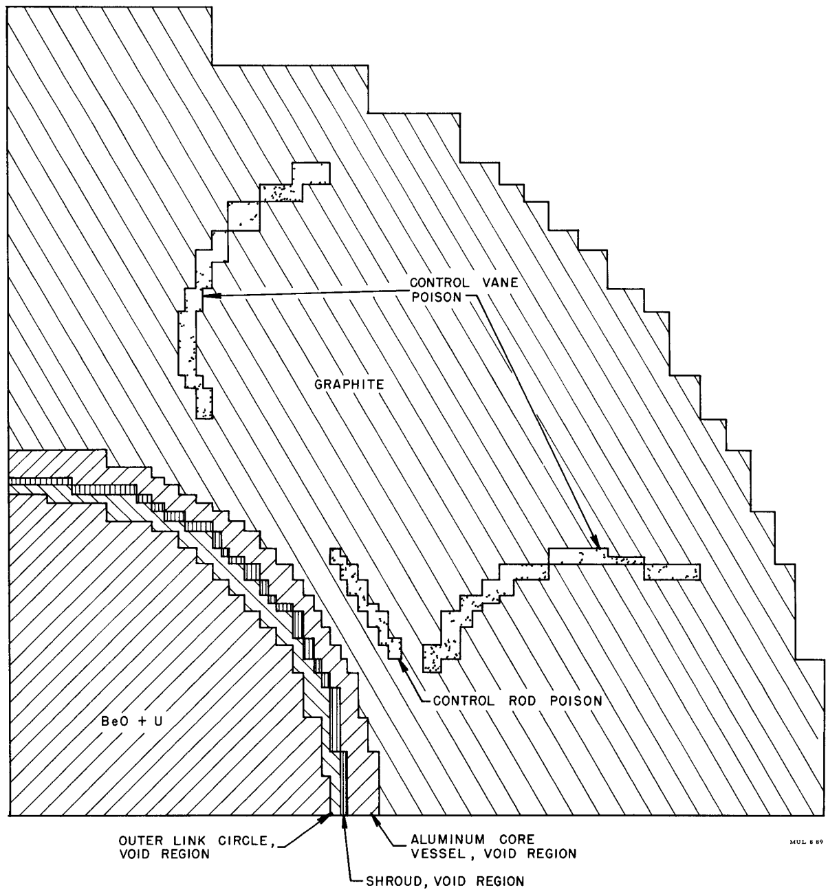
Fig. 5-1. Reactor cross section as described by neutronics code.
