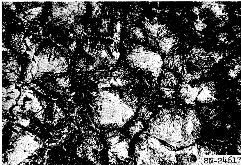
Fig. I-4. Forged Marman clamp, electro-etched after cathodic etching to bring out tempered martensite. Light area was retained austenite, subsequently transformed at NTS, darker area is the tempered martensite. (100X)
