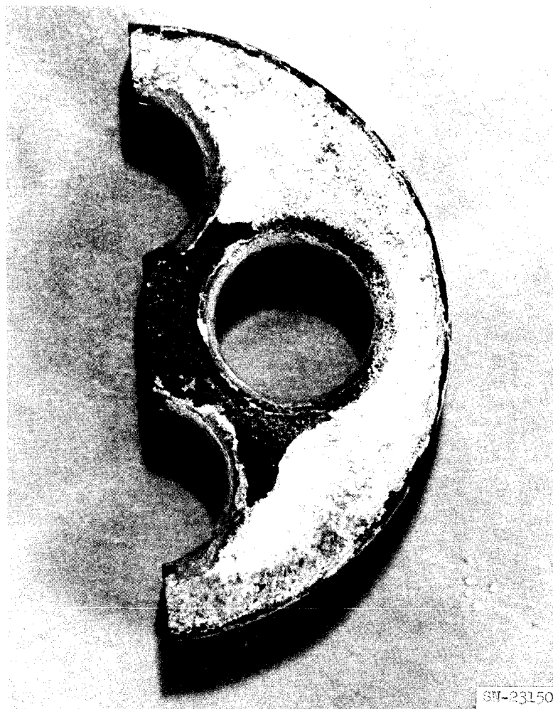
Fig. III-43. Downstream face of specimen CR after 5-hr exposure at 2275°F. Loss of coating is significantly less than on upstream face. (Mag: 4×)
