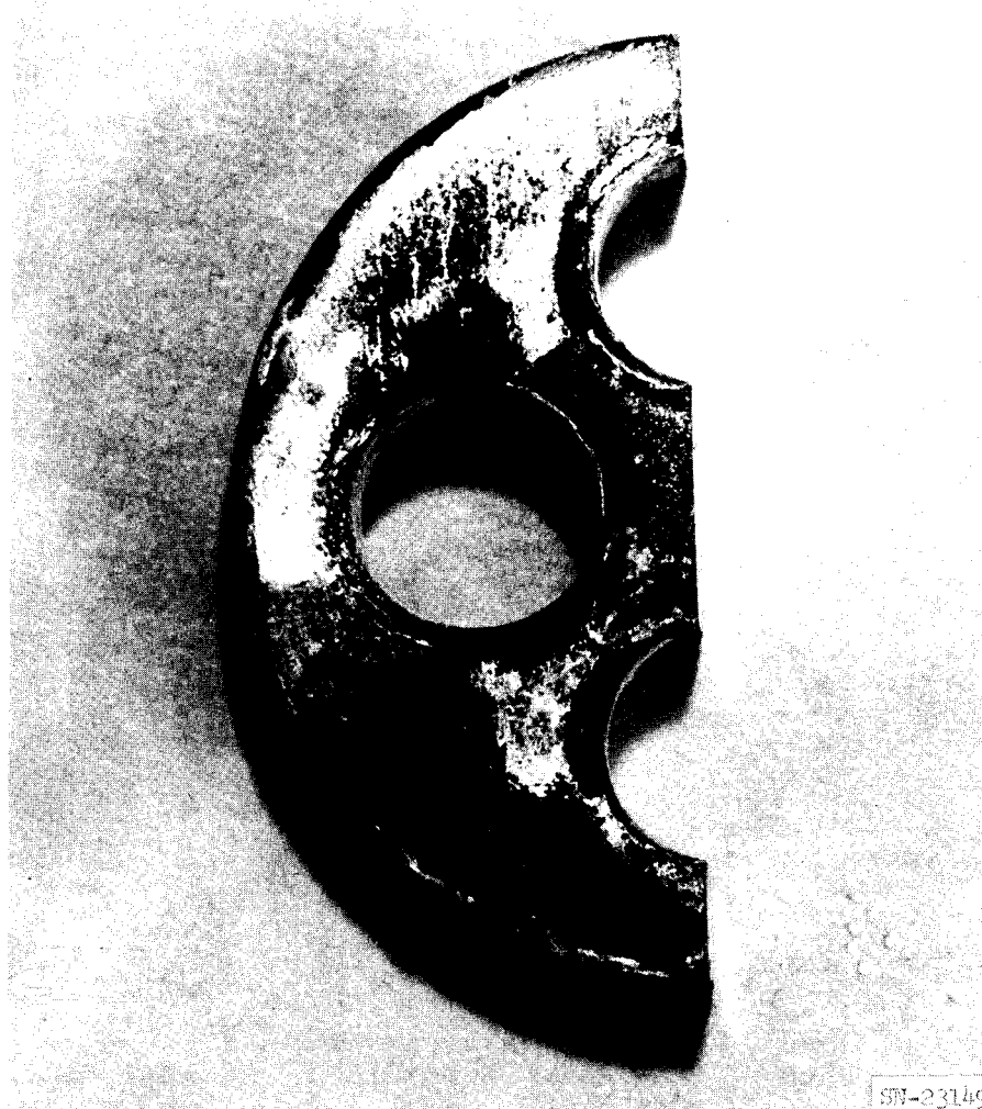
Fig. III-44. Upstream face of specimen CR after 5-hr exposure at 2275° F. Some attrition of the coating is apparent in the lower half of the specimen. (Mag: 4X)
