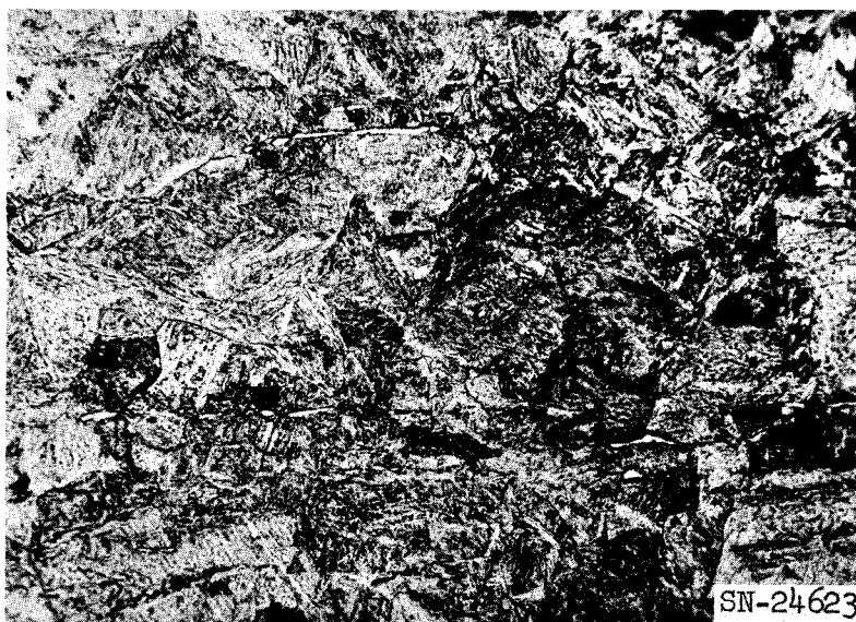
Fig. I-11. Forged AM355 Marman clamp which cracked during SCT heat treatment. Longitudinal section, cathodically etched. (100X)
