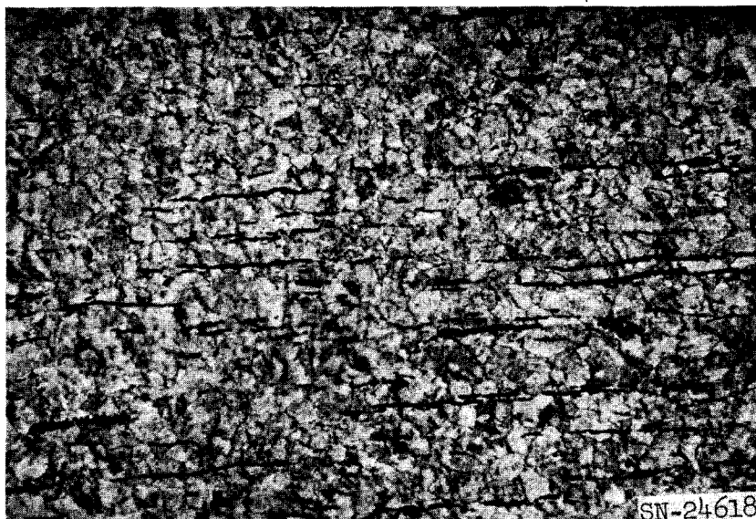
Fig. I-5. Marman clamp bolt, 100% tempered martensite. Electro-etched. (100X)
