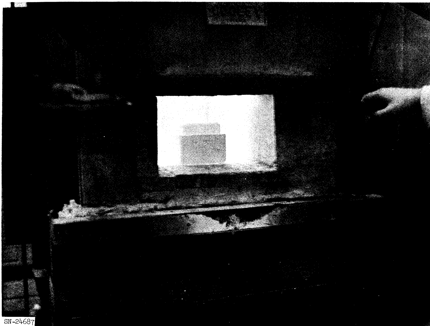
Fig. III-48. Loaded retort containing base plate and hot module flow test plate. Furnace is at 1900°F. Specimens will be processed for 16 hr as one cycle of the silicon-chromium/aluminum pack coating methods.
