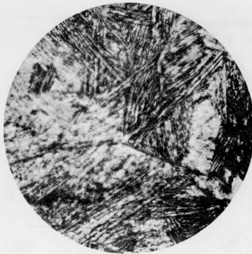
Plate 142-1-4 5 atomic % Cb. 2000X. Electrolytic polish; etched. Portions of three grains with dark constituent (Cb-rich phase) in grain boundary. Appears to be about eutectoid composition.
