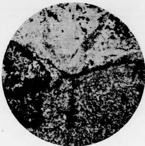
Plate 170-1-8 10 atomic % Cb. 2000X. Electrolytic polish; etched. Structure of the Cb-rich phase.
