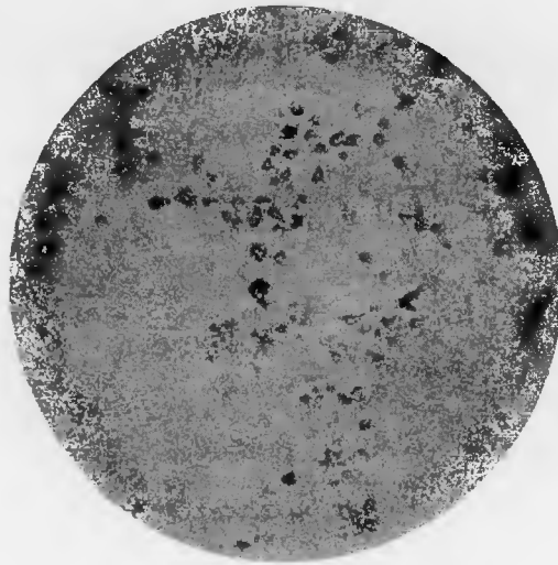
Plate 138-1-2. 0% Cb. 250X. Electrolytic polish; not etched. High concentration of carbides in Area I.
