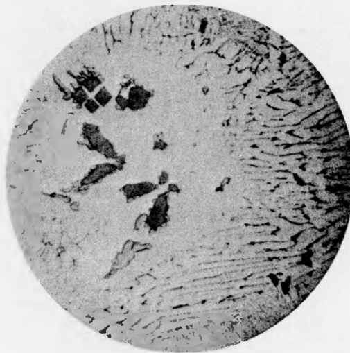
Plate J-112-1-6. 1.5 atomic % Cb. 1000X. Electrolytic polish. Shows carbides to which are attached particles of alpha ( \alpha ) phase.
