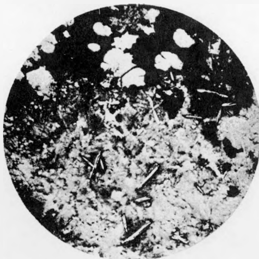
Plate 170-1-5. 10 atomic % Cb. 250X. Electrolytic polish; etched. Porous portion, Area I, shows carbides (rectangular gray) and unidentified compound (needles). Matrix is largely Cb-rich phase.
