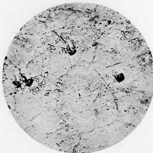
Plate 142-1-2. 5 atomic % Cb. 250X. Electrolytic polish; etched. Carbides greater in number in Area III.
