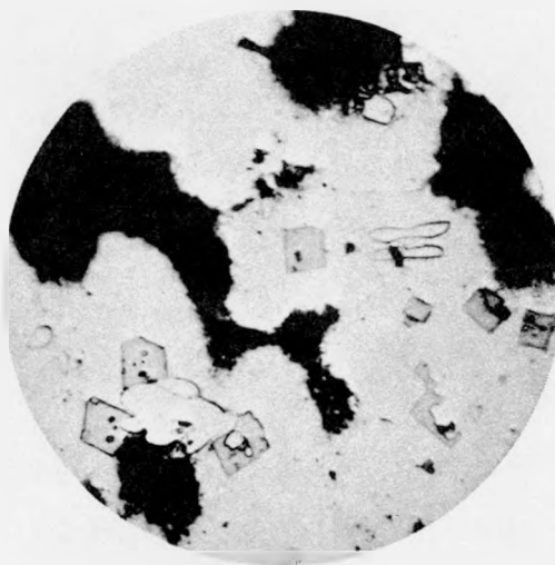
Plate 185-1-13. 20 atomic % Cb. 1000X. Electrolytic polish; etched. Carbides (gray rectangular phase) and unidentified needles.
