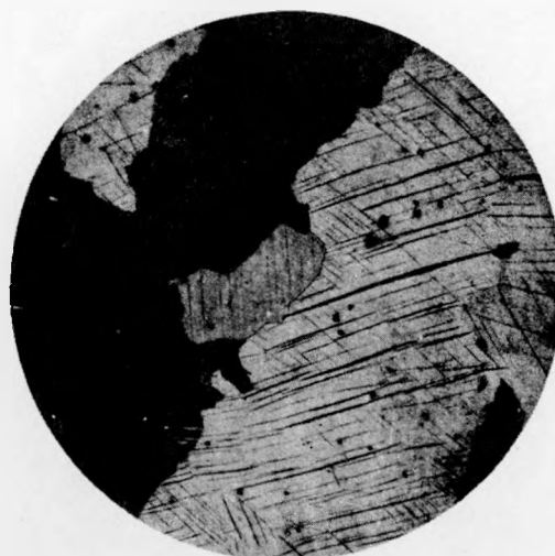
Plate 138-1-1. 0% Cb. 100X. Electrolytic polish; polarized light.
