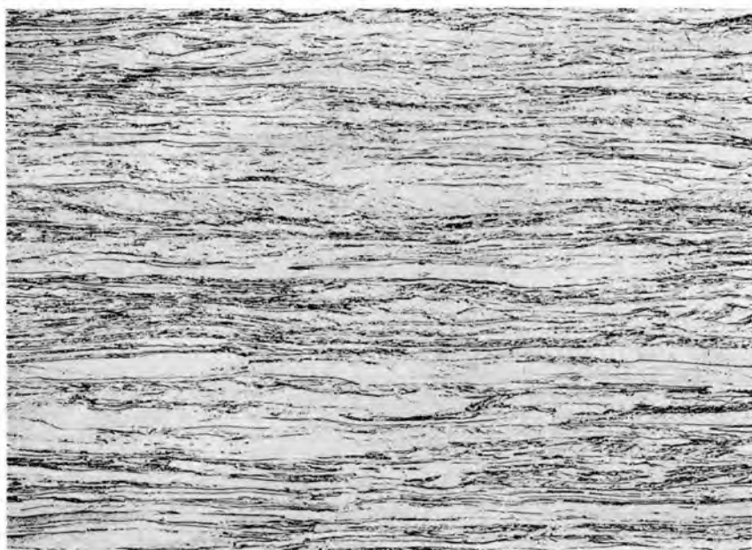
Figure 31 (Y-23129). Microstructure of 80% reduced arc-cast niobium, annealed one hour at 900°C. Etchant - 25 HF, 50 H 2 O, 5 HNO 3 , 10 H 2 SO 4 . 100X.
