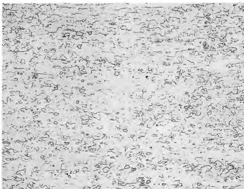
Figure 46 (Y-23157). Microstructure of 80% reduced powder-metallurgy niobium, annealed 1/4 hour at 1100°C. Etchant - 25 HF, 50 H 2 O, 5 HNO 3 , 10 H 2 SO 4 . 100X.
