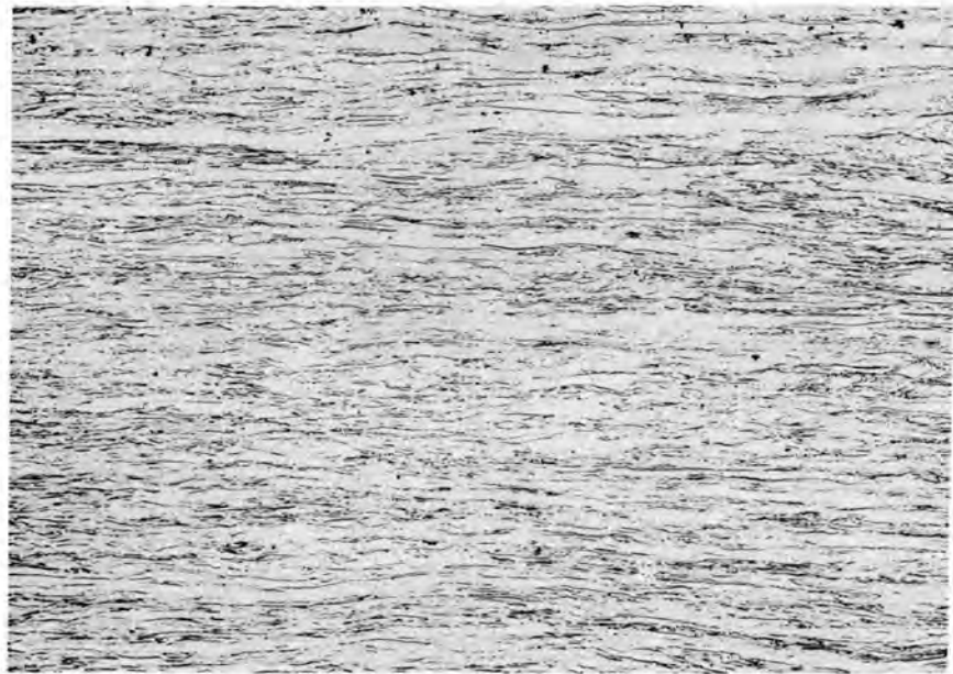
Figure 30 (Y-23134). Microstructure of 80% reduced powder-metallurgy niobium, as rolled. Etchant - 25 HF, 50 H 2 O, 5 HNO 3 , 10 H 2 SO 4 . 100X.
