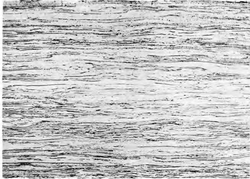
Figure 29 (Y-23124). Microstructure of 80% reduced arc-cast niobium, as rolled. Etchant - 25 HF, 50 H 2 O, 5 HNO 3 , 10 H 2 SO 4 . 100X.
