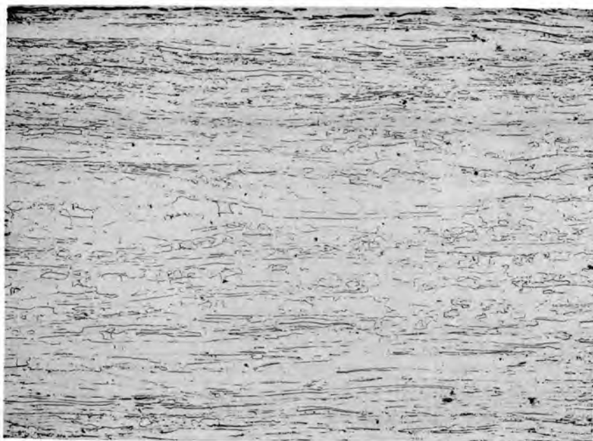
Figure 39 (Y-23142). Microstructure of 80% reduced arc-cast niobium, annealed 1/4 hour at 1000°C. Etchant - 25 HF, 50 H 2 O, 5 HNO 3 , 10 H 2 SO 4 . 100X.
