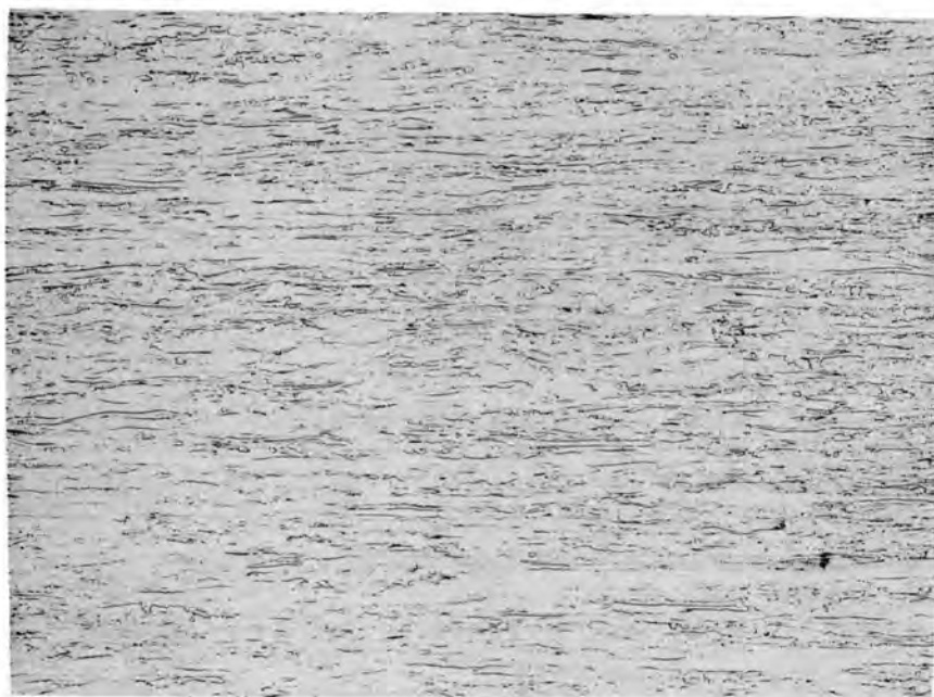
Figure 40 (Y-23141). Microstructure of 80% reduced powder-metallurgy niobium, annealed 1/4 hour at 1000°C. Etchant - 25 HF, 50 H 2 O, 5 HNO 3 , 10 H 2 SO 4 . 100X.
