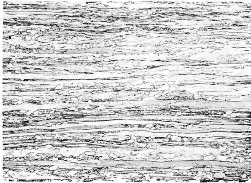
Figure 33 (Y-23128). Microstructure of 80% reduced arc-cast niobium, annealed one hour at 1000°C. Etchant - 25 HF, 50 H 2 O, 5 HNO 3 , 10 H 2 SO 4 . 100X.
