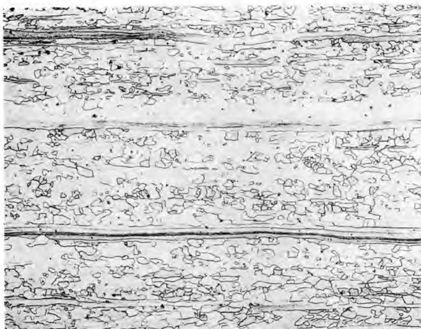
Figure 47 (Y-23158). Microstructure of 80% reduced arc-cast niobium, annealed two hours at 1100°C. Etchant - 25 HF, 50 H 2 O, 5 HNO 3 , 10 H 2 SO 4 . 100X.
