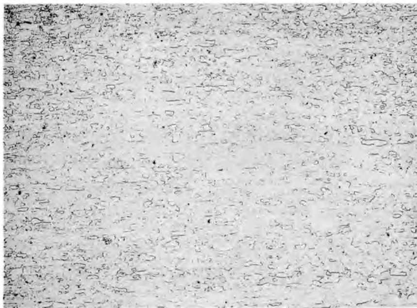
Figure 44 (Y-23139). Microstructure of 80% reduced powder-metallurgy niobium, annealed ten hours at 1000°C. Etchant - 25 HF, 50 H 2 O, 5 HNO 3 , 10 H 2 SO 4 . 100X.
