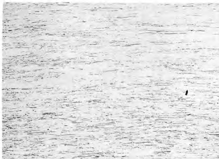
Figure 32 (Y-23133). Microstructure of 80% reduced powder-metallurgy niobium, annealed one hour at 900°C. Etchant - 25 HF, 50 H 2 O, 5 HNO 3 , 10 H 2 SO 4 . 100X.
