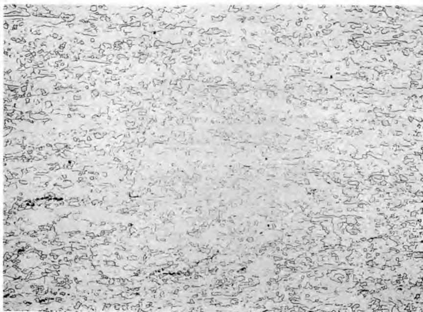
Figure 10 (Y-23136). Typical microstructure of powder-metallurgy niobium, parallel direction. Etchant - 25 HF, 5 H 2 O, 5 HNO 3 , 10 H 2 SO 4 . 75X.
