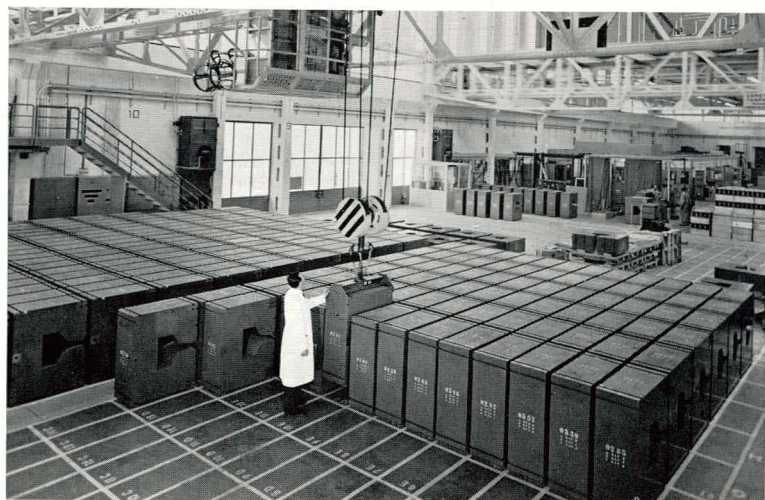
Unloading of a magnet block on delivery and placing it in position for storing.
