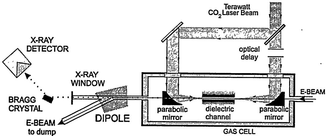
Fig.1 Principal diagram of the compact LSS based on laser wakefield acceleration in a waveguide;
