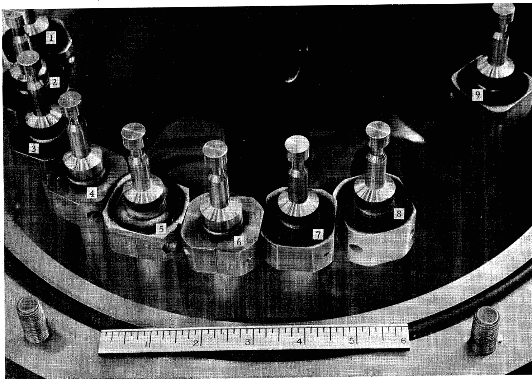
Fig. 18. Black Soot-Like Deposit Around Welds and Chill Blocks
