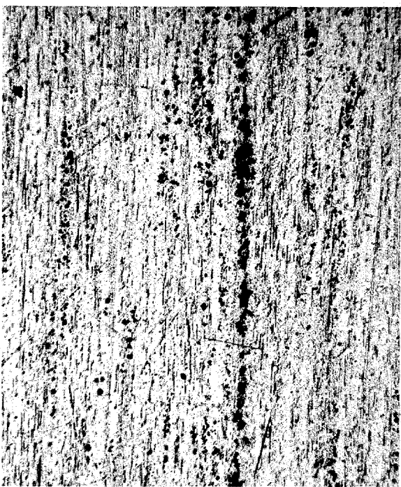
28-20F Transverse section End section of last slug in rod Many strung out oxides and void areas strung out with the oxides 50X
