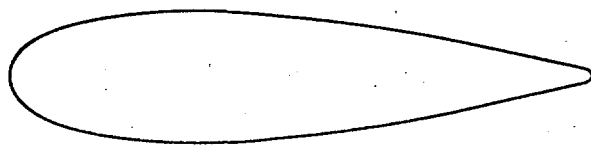
Root Section - 121.9cm Chord NACA 0021
