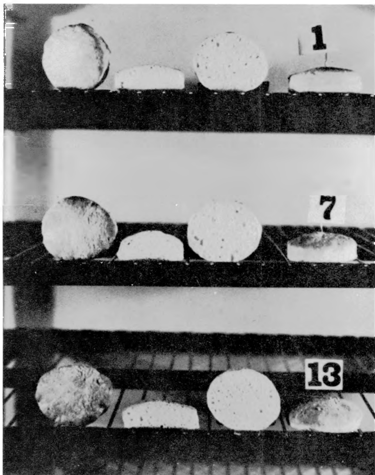
Fig. 37 — Comparison of baking powder biscuits made from prepared biscuit flour exposed in trench at 1270 ft (1), in house at 7800 ft, (7), and biscuits made from unexposed flour (13). No difference in baking quality noted.
