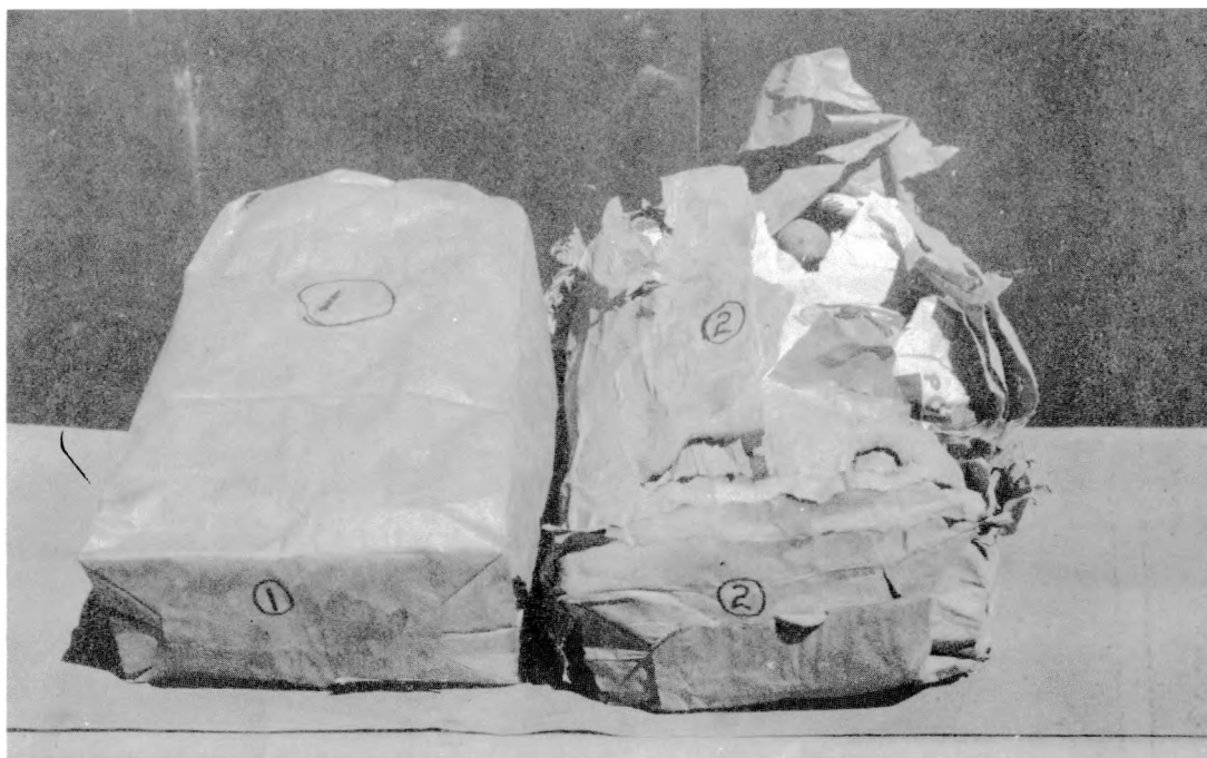
Fig. 17—Physical damage to multiwall kraft bag of potatoes buried flush with ground with no soil cover at Station A (1100 ft) (right). Check bag not exposed (left).
