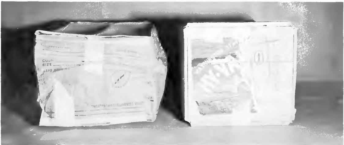
Fig. 18—Blast caused greater damage to fiberboard box than to wooden box of apples in trench at Station A (1270 ft), but bruising was severe in both types of container.
