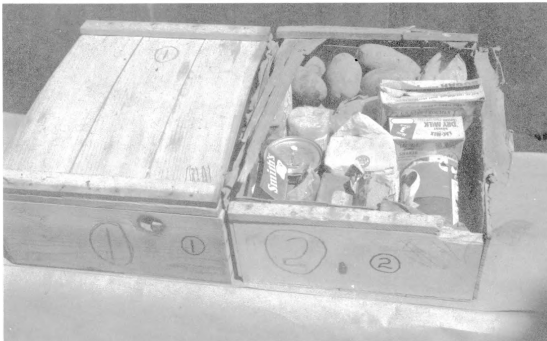
Fig. 16—Box buried flush with ground with no soil cover at Station A (1100 ft) (right). (Note destruction of cover and loss of polyethylene potato bag.) Check box not exposed (left).
