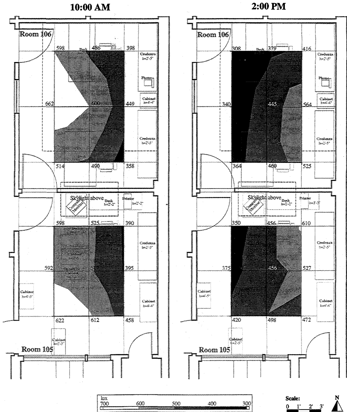
Figure 5. Workplane illuminance (lux) in Rooms 105 and 106 at 10:00 AM and 2:00 PM
