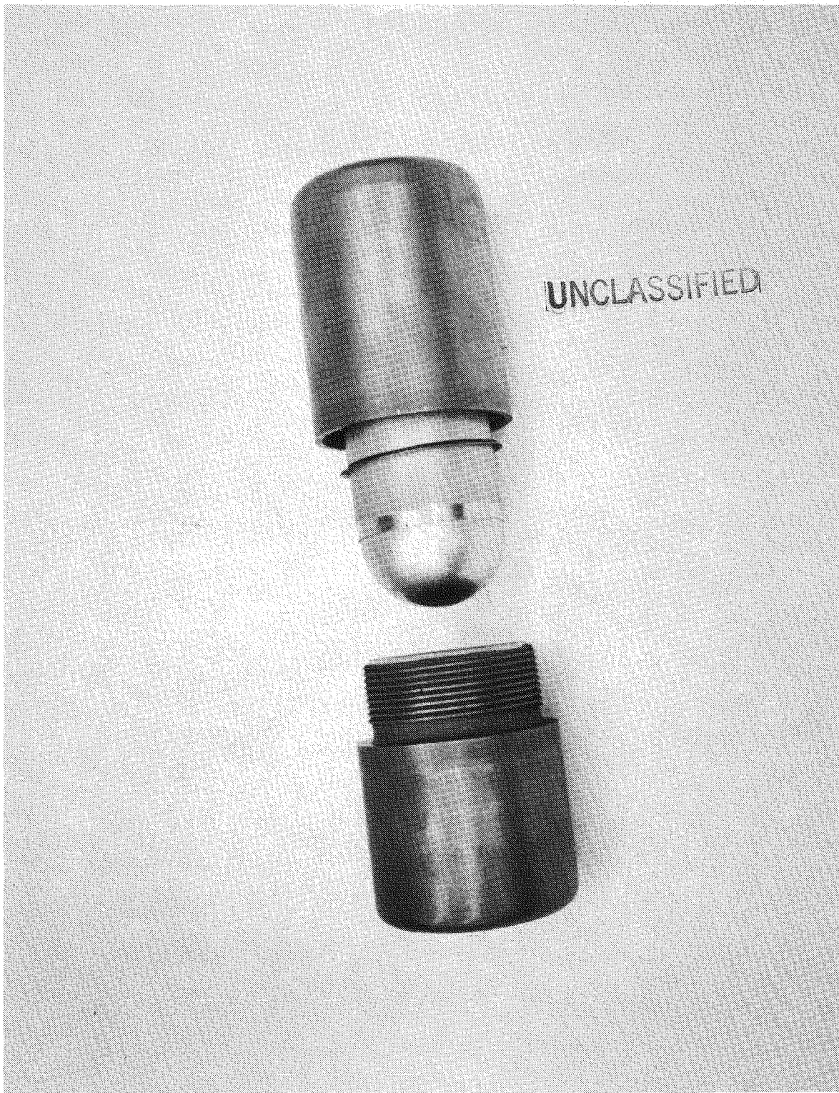
FIGURE 23 - Graphite heat shield showing canistered SNAP-19B (IRHS) capsule in female section.
