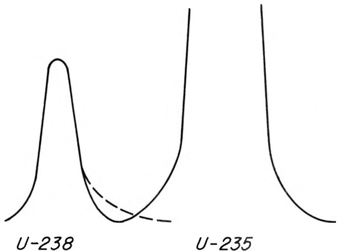
*Dotted Line Shows Possible Condition When Impurities Are Present In Enriched Uranium. The Toe Of The U-238 Peak Contributes To The U-235 Peak.*
