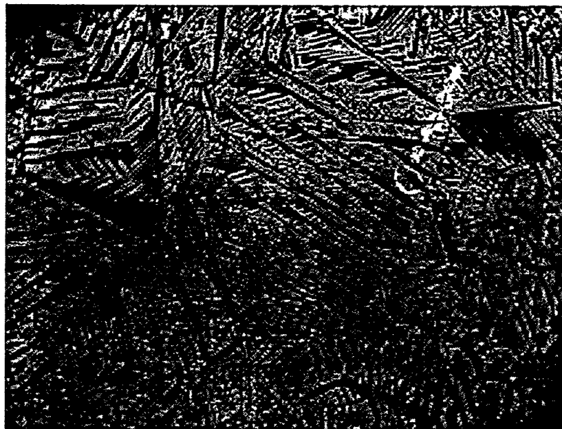
Figure 1.10 Backscatter Image: Phase Separation Exhibited
