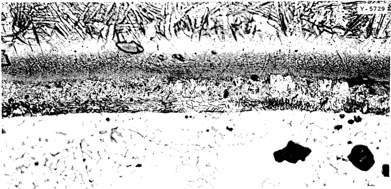
Fig. 113. Microstructure of the Plate Rolled with a Reduction of 30:1 After Heat Treatment for 2 min at 1075°C in Vacuum. Etched with acetic and perchloric acids. 1000X.
