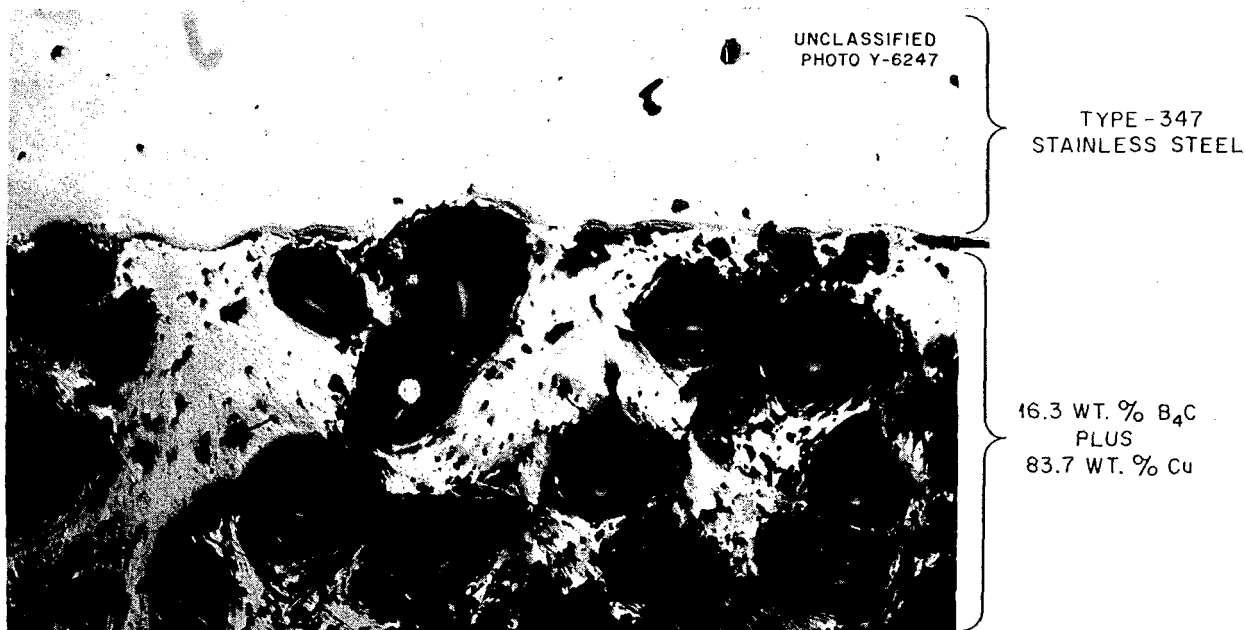
Fig. 67. Interface of Type-347 Stainless Steel Cladding and Copper-Boron Carbide Core. 200X. Reduced 18%.
