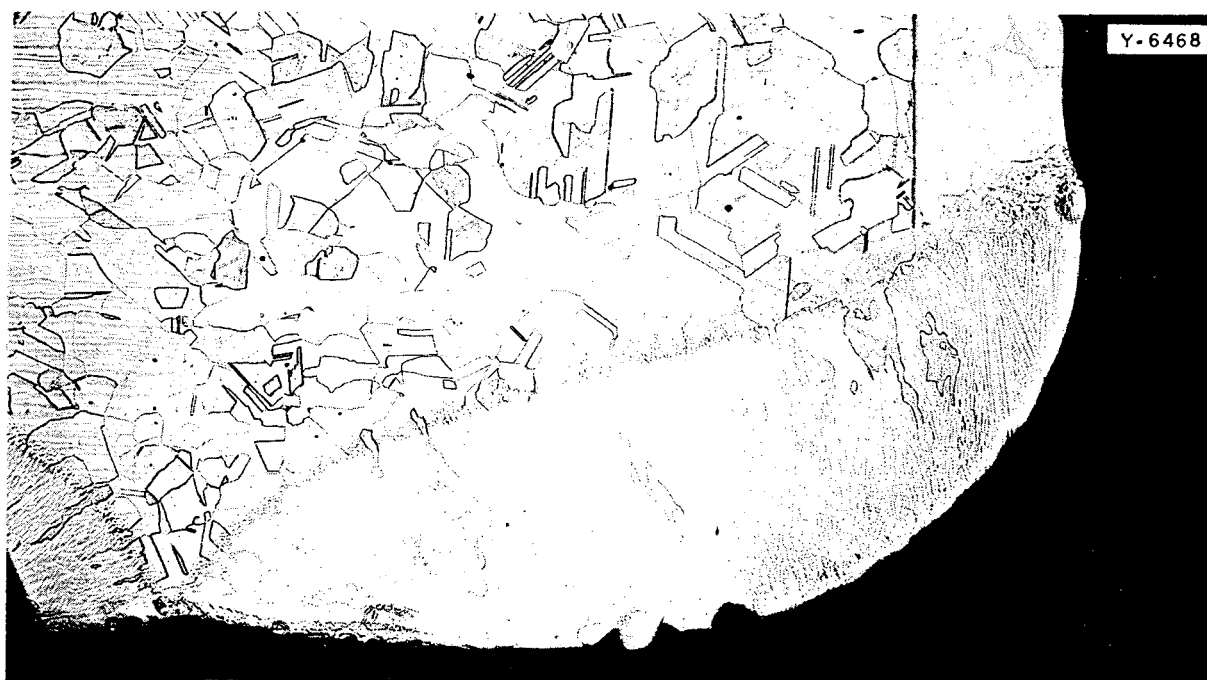
Fig. 66. Transverse Section of a Typical Tube-to-Header Cone-Arc Weld of 1/8-in. Type-304 Stainless Steel Header Sheets and Type-316 Stainless Steel Tubes, 0.10 in. OD, 0.010-in. Wall Thickness. 10X.
