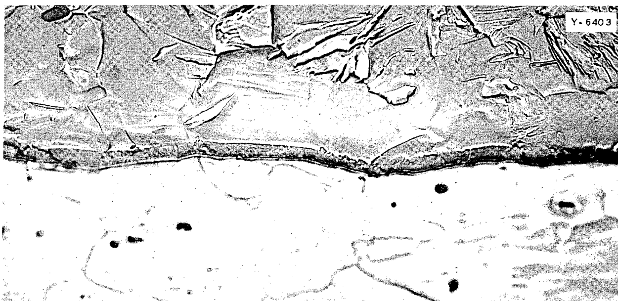
Fig. 107. Microsturcture in the Bond Area of a Plate Rolled from a Billet that Was Evacuated, Helium Flushed, and Re-evacuated Before Sealing. Etched with acetic and perchloric acids., 1000X.
