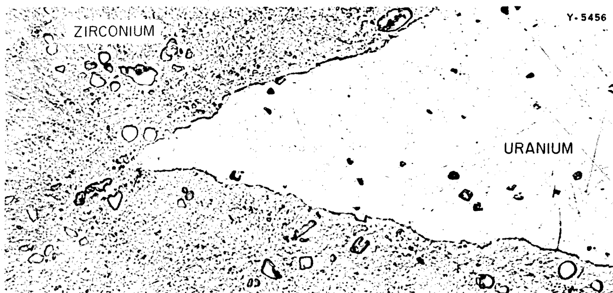
Fig. 91. Bonding at Edge of Uranium-Zirconium Plate. Etched with acetic and perchloric acids. 500X.
