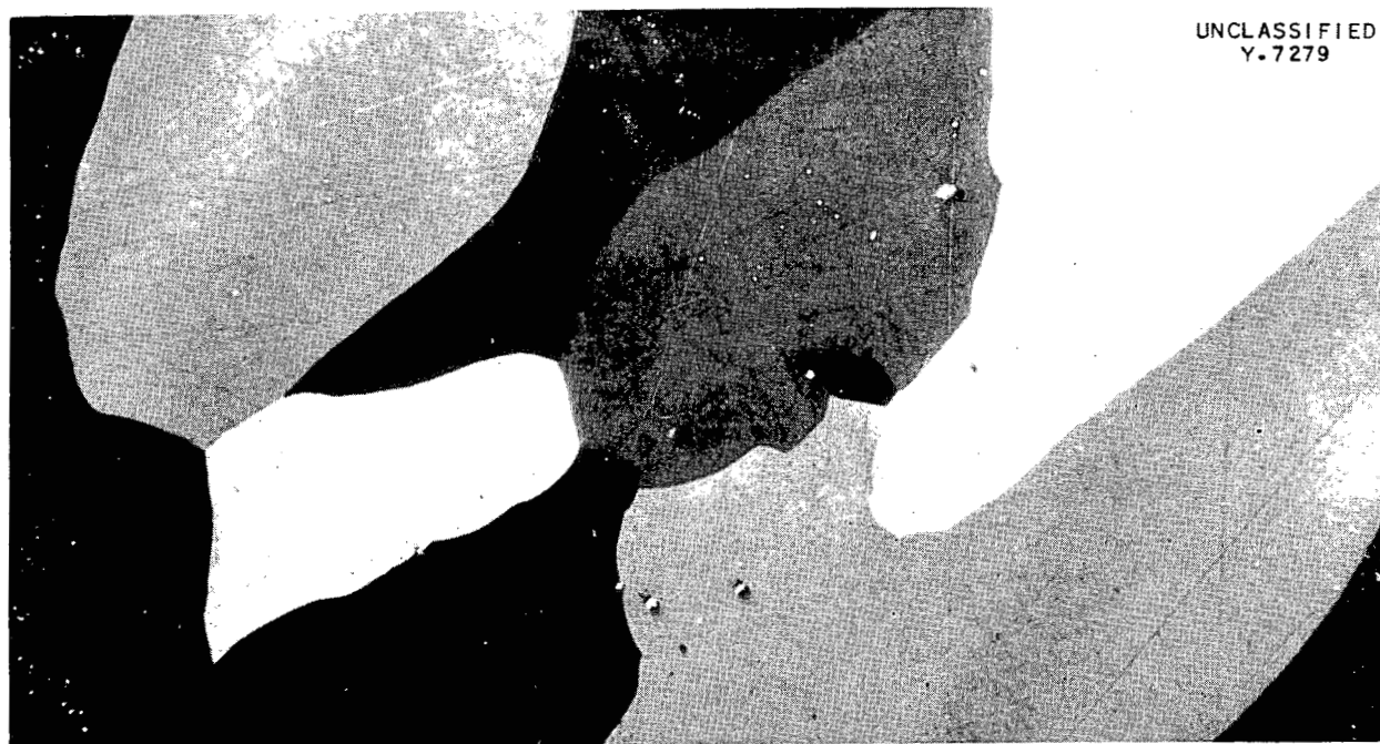
Fig. 14. Alloy 48.3 Annealed Ten Days at 779°C Showing the AgZr Phase with a Small Amount of Silver Solid Solution. Etched briefly in 1% HF-49% acetic acid-50% glycerine; bright field. 250X
