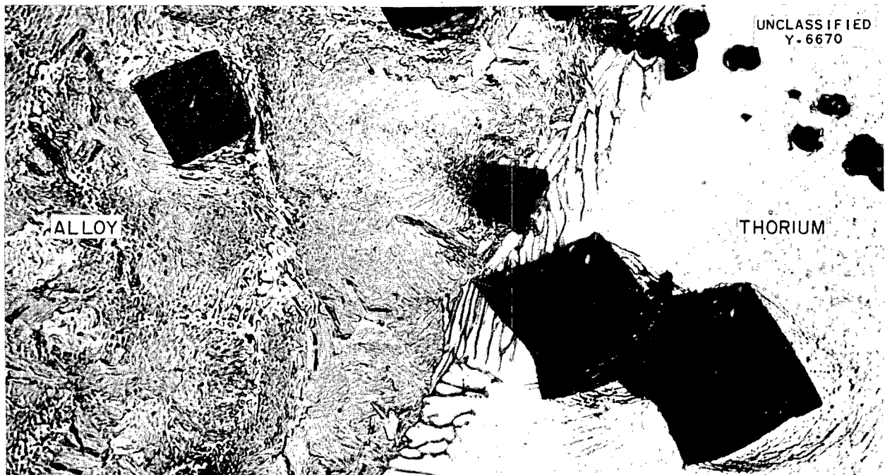
Fig. 4. As-Brazed Interfaces of Thorium Billet Brazed to Zirconium with 73% Thorium-22% Zirconium Alloy. Etched with perchloric and acetic acids. 500X
