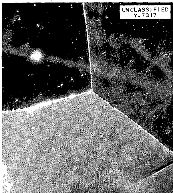
Fig. 15. Indium-Zirconium Alloy 9.6 Annealed for 96 hr at 972^\circ\text{C} Followed by Annealing for Nine Days at 847^\circ\text{C} Showing Isothermal Alpha Phase. Etched with 20% HF-20% \text{HNO}_3 -60% glycerine; polarized light. 250X
