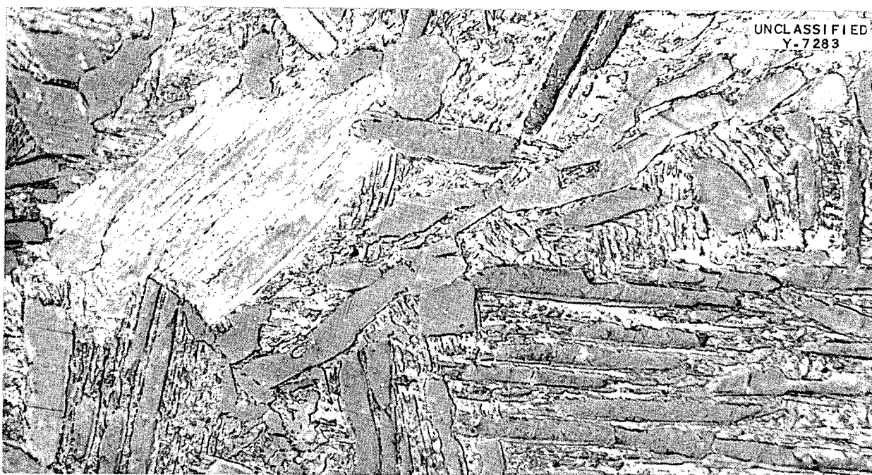
Fig. 9. Alloy 0.51 Quenched from 857.4°C Showing the Two-Phase Microstructure with Large Grains of Alpha Phase in a Matrix of Decomposed Beta Phase. Etched with 0.5% HF-50% alcohol-49.5% glycerine mixture; polarized light. 250X
