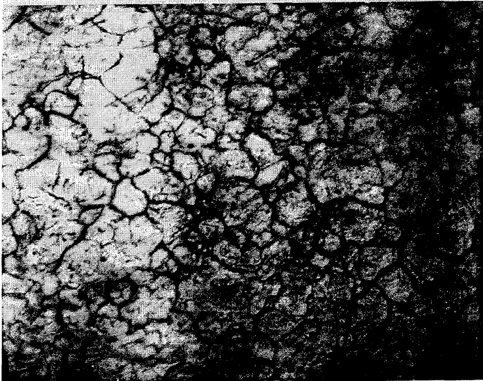
Figure 1. Type 304L stainless steel before polishing (500x magnification).
