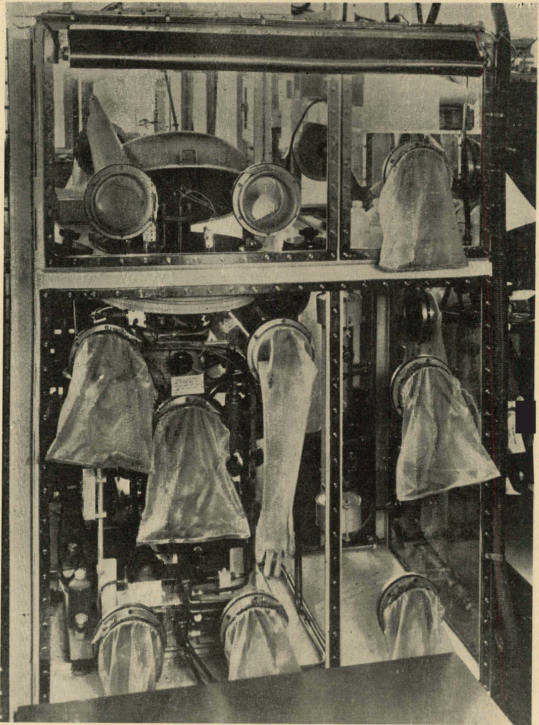
FIGURE 2:—Showing free-standing alpha-active box for metal casting.
