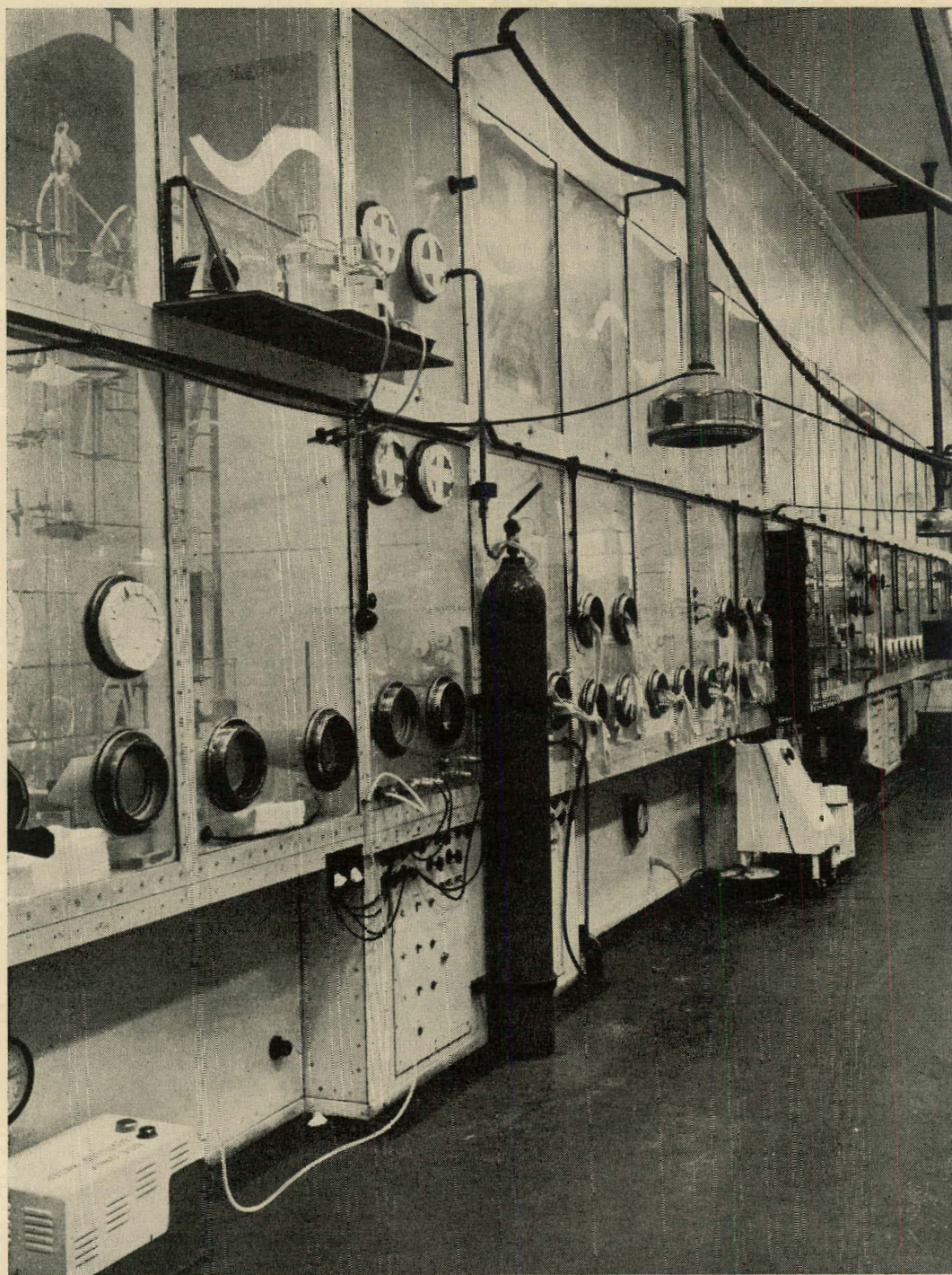
FIGURE 1:—Showing length of block fixed boxes for plutonium metallurgical researches.
