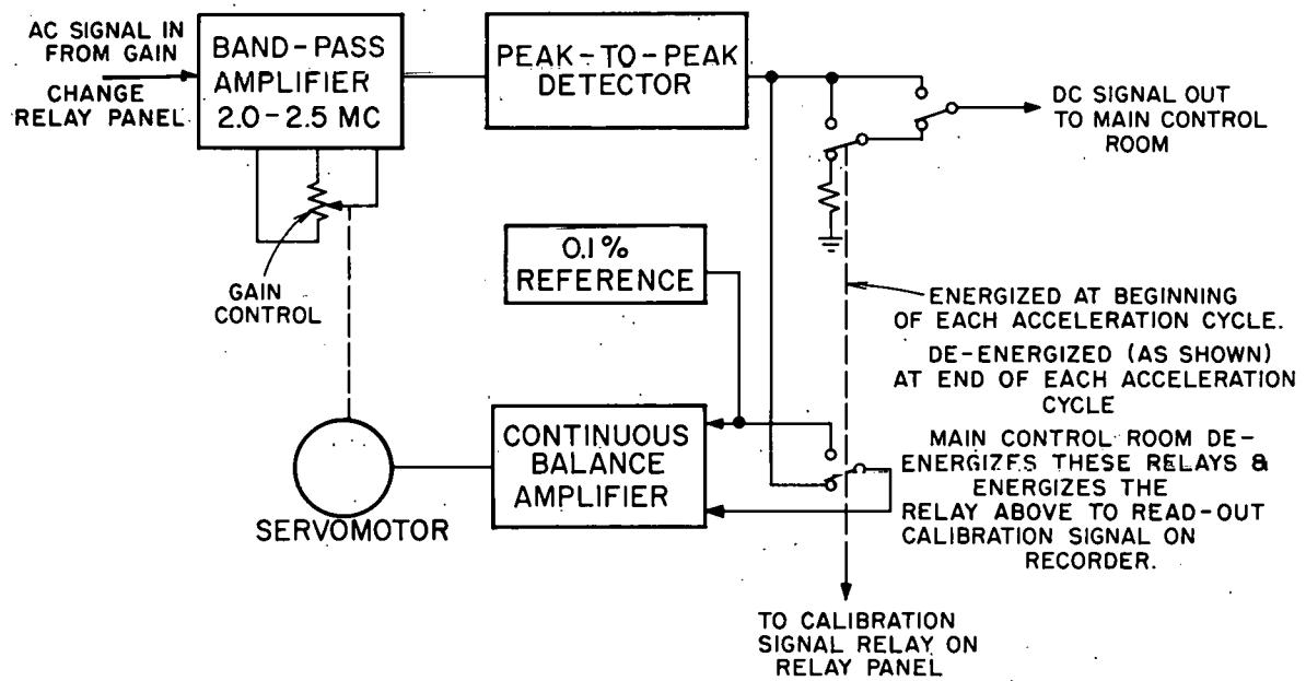
Fig. 5. Bevatron east induction-electrode system--band-pass amplifier and peak detector.
