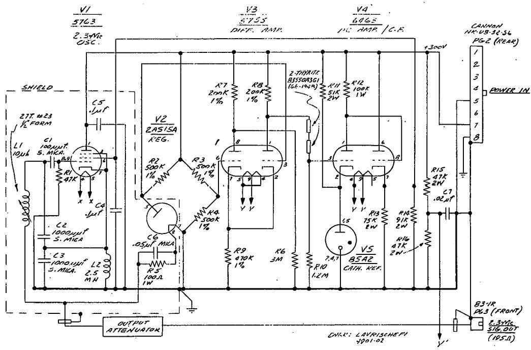
Fig. 10. Calibration-signal generator.
