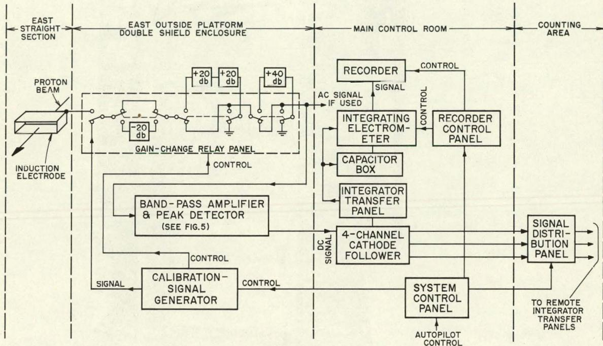
Fig. 2. Bevatron east induction-electrode system (block diagram)
