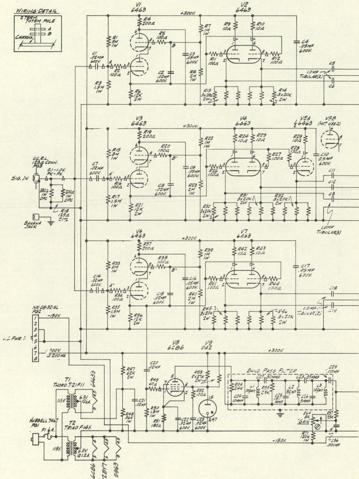
Fig. 8. Bevatron south induction-electrode system: band-pass amplifier, peak detector, and 7-channel cathode follower.
