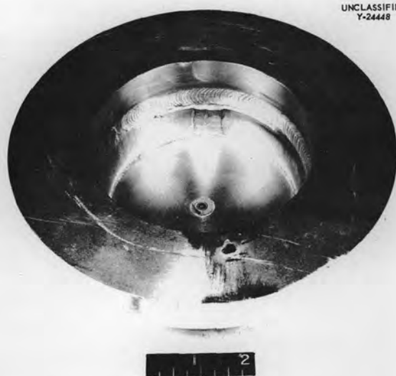
Fig. 2.1.34. Bottom View of Completed Pump Fabrication Test Assembly.
