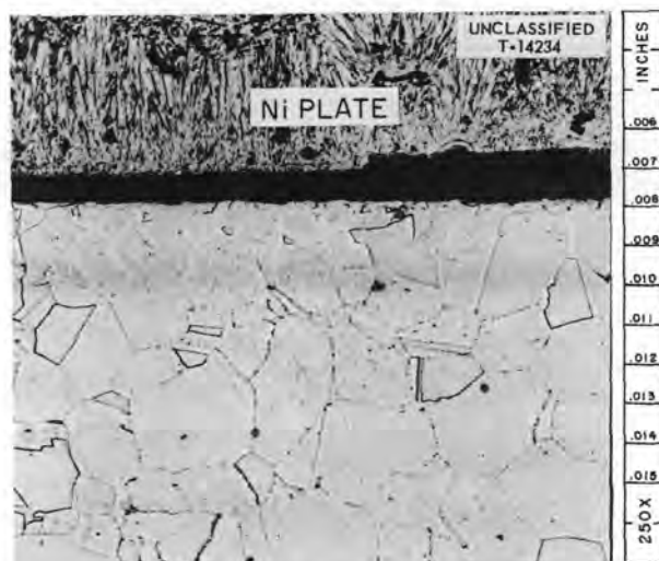
Fig. 2.1.6. Section Taken from Inconel Forced-Circulation Loop CPR at Discharge End of Heated Leg. 250X. Reduced 22%.
