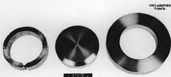
Fig. 2.1.32. Pump Fabrication Test Components Prior to Welding.
