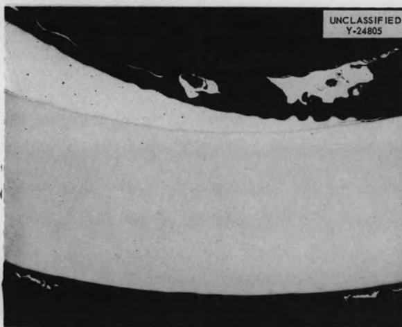
Fig. 2.1.18. Specimen Showing Excellent Wetting of a Nickel Tube by Silver. Unetched. 50X. Reduced 30%.
