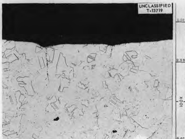
Fig. 2.1.37. Specimen Showing Lack of Fusion Found in Weld Area of INOR-8 Tubing. Etchant: aqua regia. 100X. Reduced 31%.
