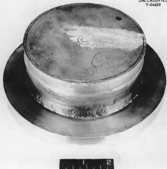
Fig. 2.1.33. Top View of Completed Pump Fabrication Test Assembly.
