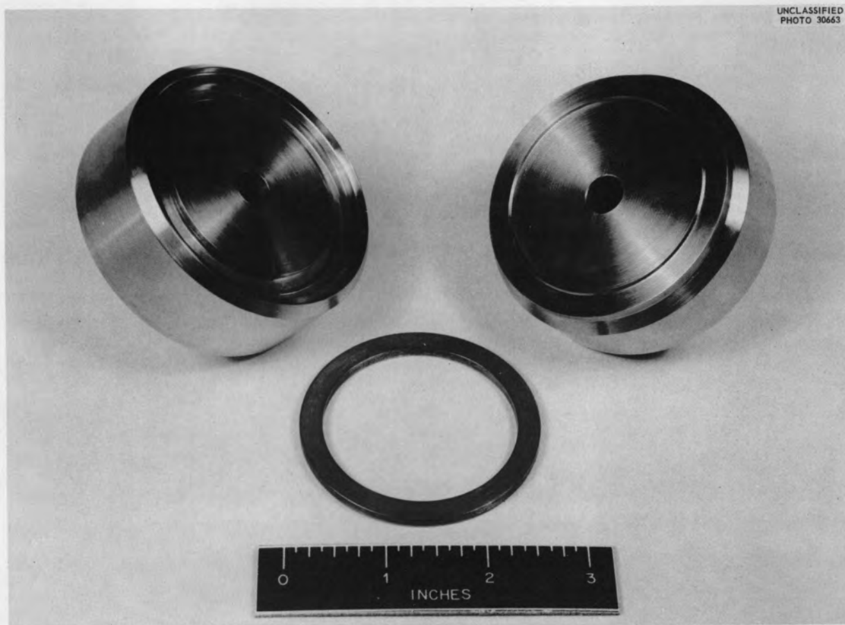
Fig. 1.2.9. Components of an Indented-Seal Flange Joint.
