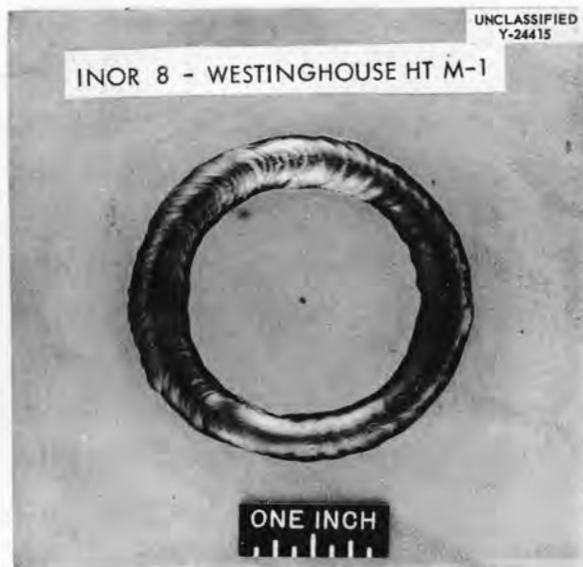
Fig. 2.1.21. Westinghouse 8M-1 Circular-Groove Weld-Cracking-Test Specimen.
