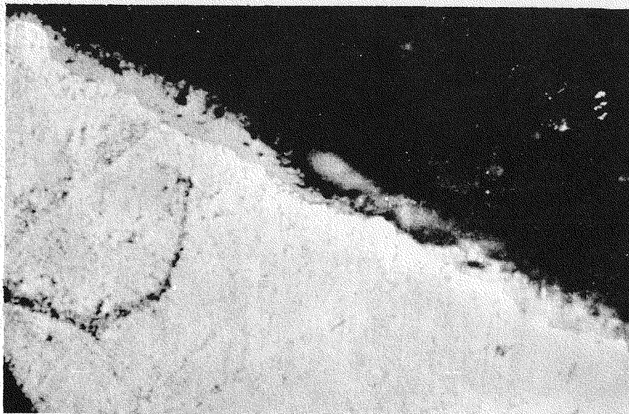
FIG. 23: \text{ZrO}_2 film at interface of \text{UO}_2 and Zircaloy-2 cladding of Specimen No. 4 from Sixth Chalk River \text{UO}_2 Defect Test.
