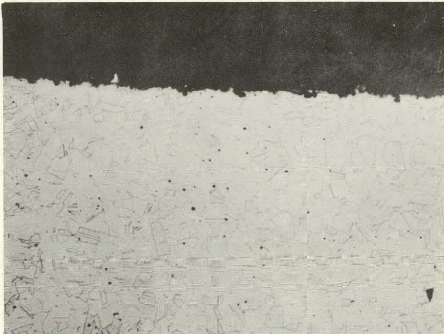
FIG. 8 PHOTOMICROGRAPH OF TYPE 304 SS PIPE SAMPLE AFTER 1200 HOURS EXPOSURE X100 OXALIC ACID ETCH
