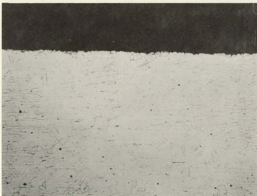
FIG. 7 PHOTOMICROGRAPH OF ORIGINAL TYPE 304 SS METAL COUPON X100 OXALIC ACID ETCH
