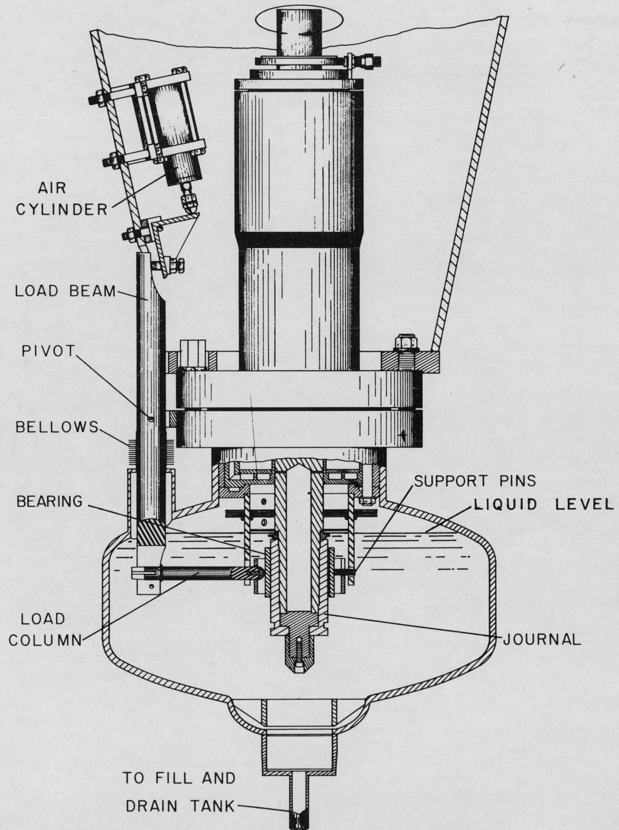
Hydrodynamic Bearing Tester, Section
